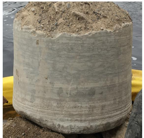
Scour occurs much more gradually in limestone bedrock – shown in this core sample taken near the US-2 bridge over the Escanaba River – than in sandy soil. To account for this variation, MDOT is developing a more precise approach to scour design customized to Michigan's surface geology.
