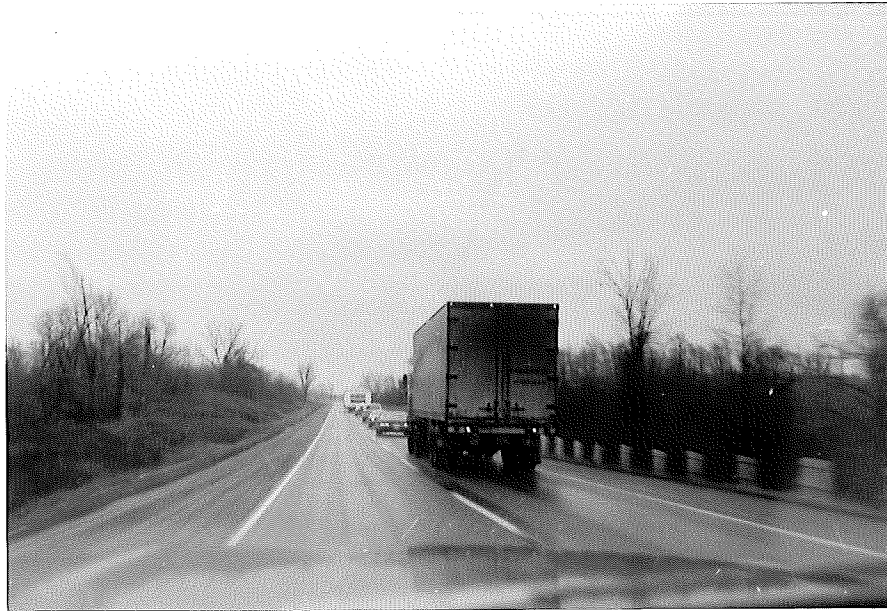
Back up of vehicles following 14-ft wide unit (US-131 S. of Three Rivers - 22-ft roadway)
