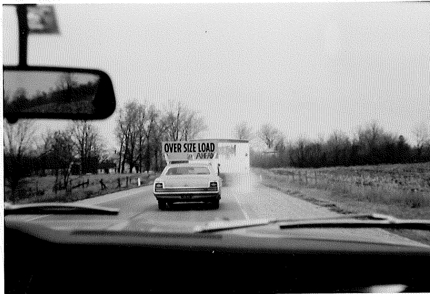
14-ft wide unit being hauled with two wheels in center of shoulder area to avoid rut at edge of roadway (US-131 S. of Constantine - 20-ft roadway)
