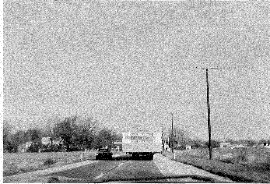
14-ft wide unit forcing approaching passenger vehicle onto shoulder (US-131 S. of Constantine - 20-ft roadway)
