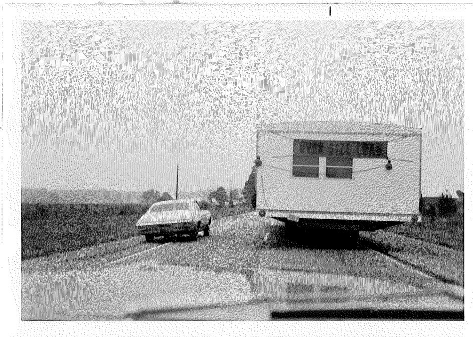
14-ft wide unit forcing trailing passing vehicle onto shoulder (note right trailer wheel in rut on edge of pavement) (US-131 S. of Constantine - 20-ft roadway)
