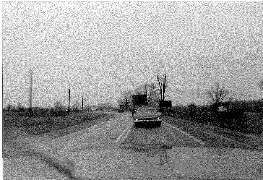
Back up of vehicles following 14-ft wide unit (US-131 S. of Three Rivers - 22-ft roadway)
