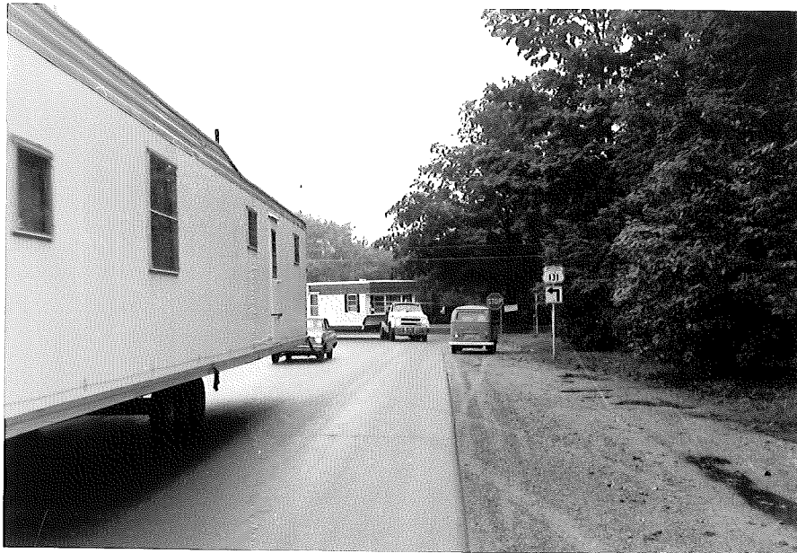
14-ft wide units forcing a vehicle onto the shoulder area (US-131 Village of Constantine - 20-ft roadway)
