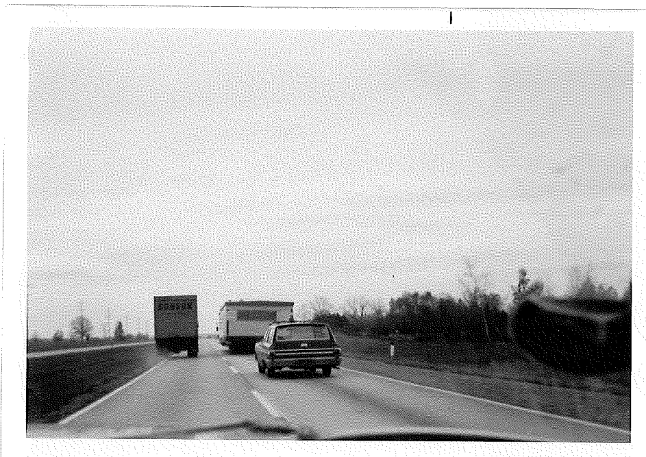
14-ft wide unit forcing trailing passing vehicle onto shoulder on 4-lane divided roadway (US-131 North of Three Rivers)
