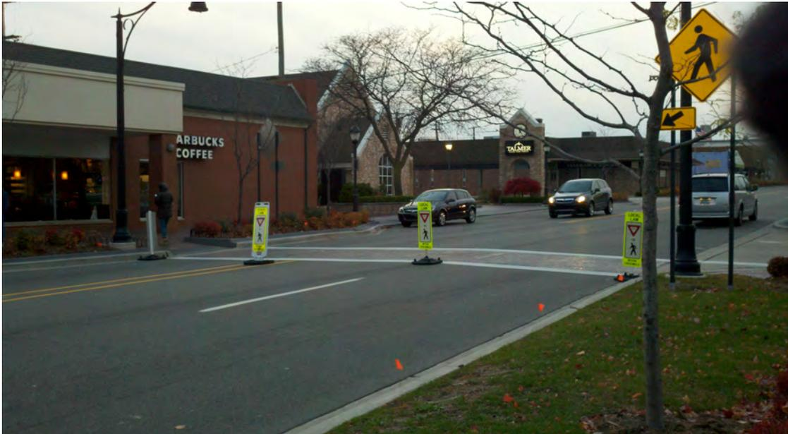
Figure a. A picture of a Gateway configuration of R1-6 signs.
