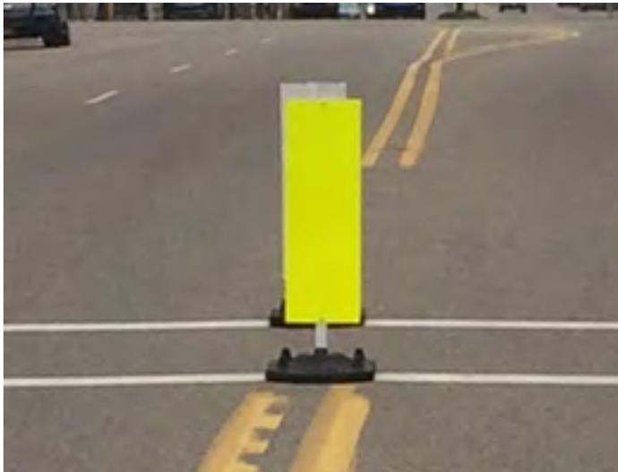
**Figure 1-3: A blank sign the same size as the R1-6 Sign mounted to a removable base**
