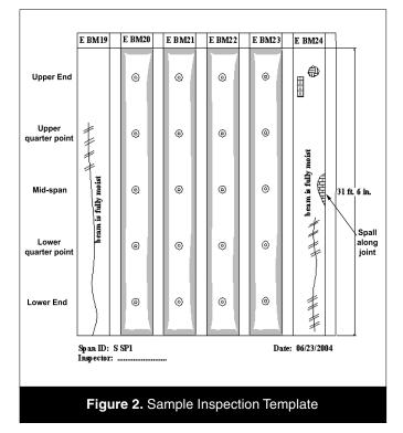
All forms of concrete distress (cracks, corrosion, spall, etc.) need to be included in the inspection by drawing the length, location, and orientation on the inspection template. The presence of rust stains or efflorescence, or the evidence of differential movement on either side of the crack should be indicated. When reporting cracks, the length, width, location, and orientation (horizontal, vertical, or diagonal) should be noted.
