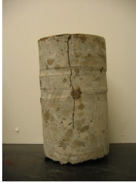
Figure 2.8. Partial-depth cracking (field core, Section A, 9-2006, station # 385+623, truck lane)
