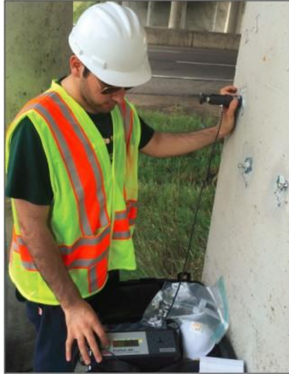
Figure 6.7 –Adhesive bond testing using PosiTect AT-A Automatic Adhesion Tester
