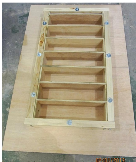
Figure 5.2.1 – Typical plywood mold assembly
