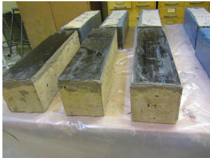
Figure 5.3.2 – FRP strengthened samples for flexure using FRP plates (sheets)
