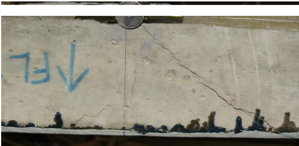
Figure 5.4.7b – Control sample 103 shear crack
