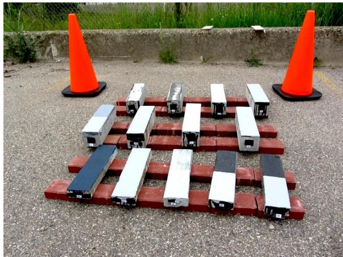
Figure 5.3.7 – Outdoor samples exposed to natural weathering
