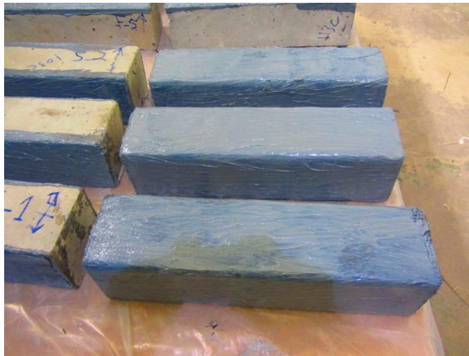
Figure 5.3.4 – FRP strengthened samples using U-wrap
