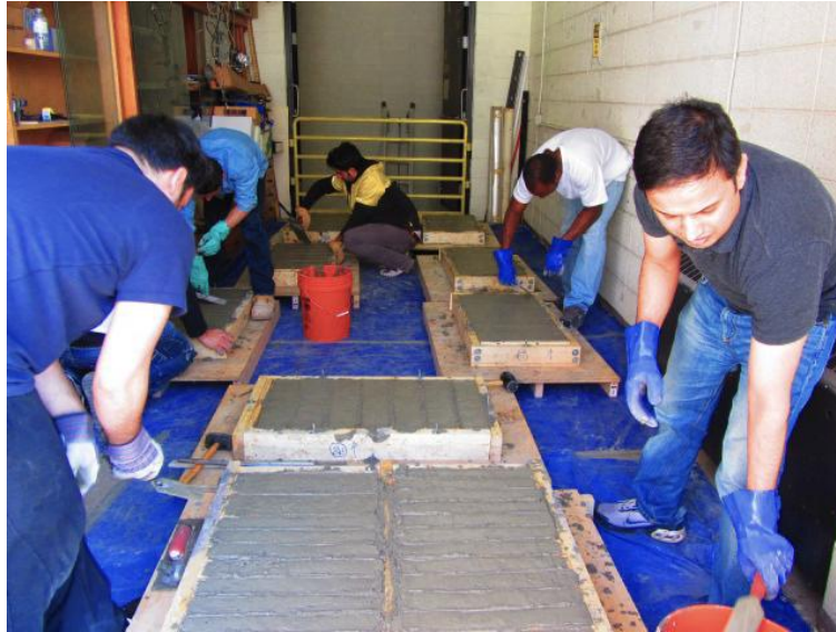
Figure 5.2.2 – Fresh concrete surface finishing
