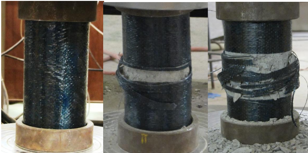
Figure 5.4.11 –Confinement sample 119 failure due to FRP rupture
