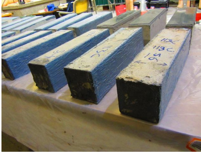
Figure 5.3.3 – FRP strengthened samples for 2-sided shear
