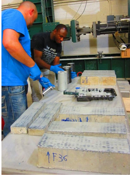
Figure 5.2.5 – FRP installation using Fyfe FRP system
