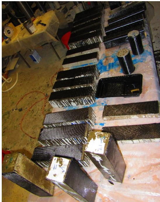
Figure 5.2.6 – Installed FRP system
