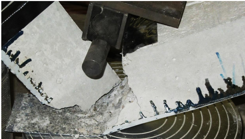
Figure 5.4.4d –Accelerated sample 101 peeling failure
