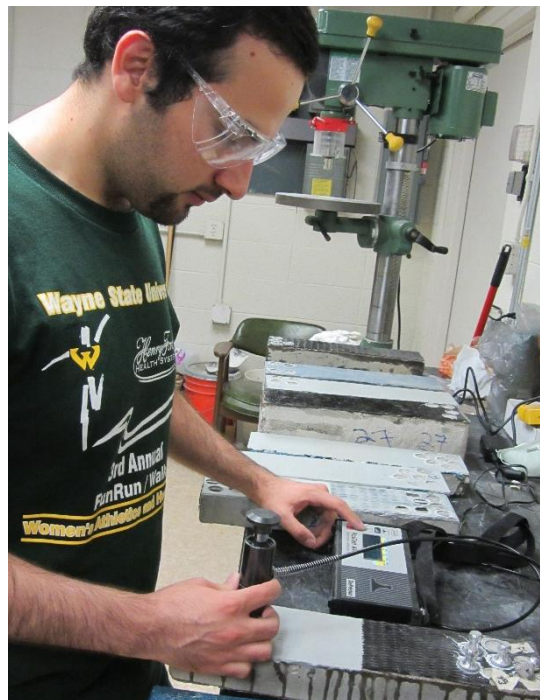
Figure 5.3.12 – Pull-off adhesion testing underway
