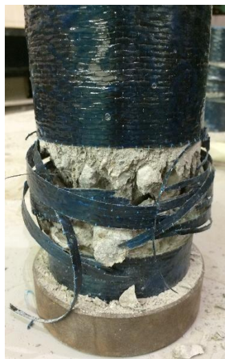
Figure 5.4.12 –Confinement sample 120 failure due to FRP rupture
