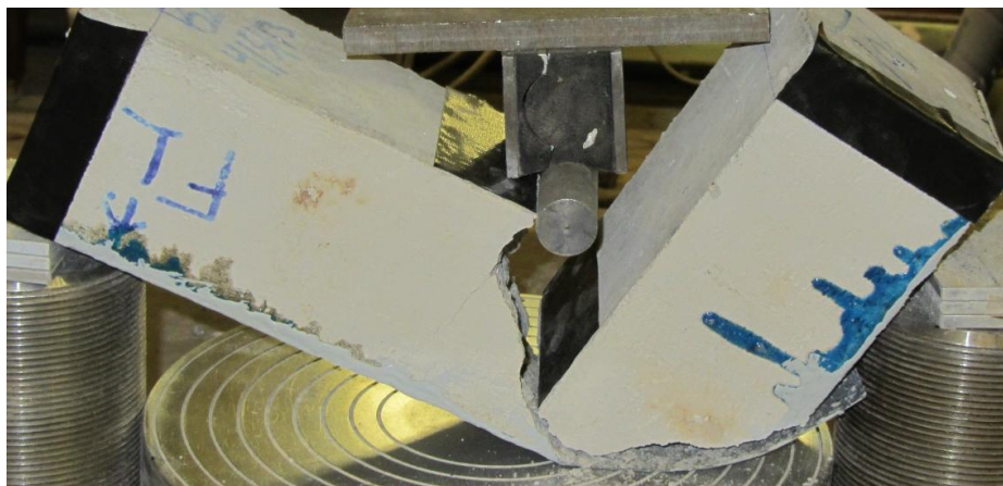
Figure 5.4.8c –Control sample 104 (shear/debonding)
