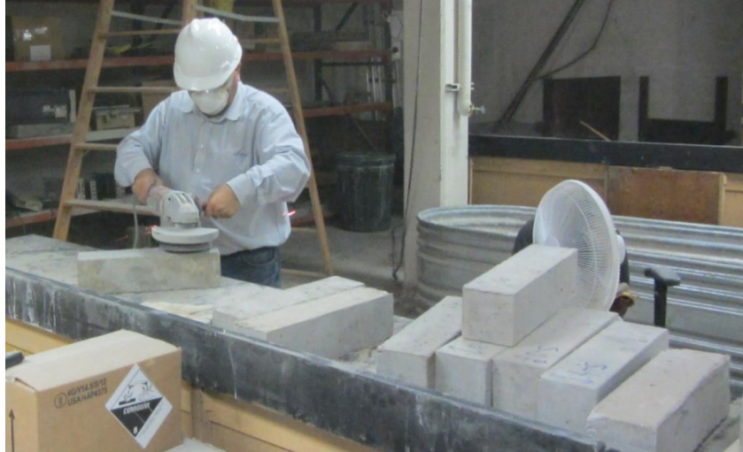
Figure 5.2.4 – Surface grinding of concrete samples
