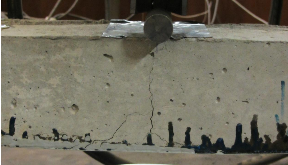
Figure 5.4.4c –Accelerated sample 101 initial cracking
