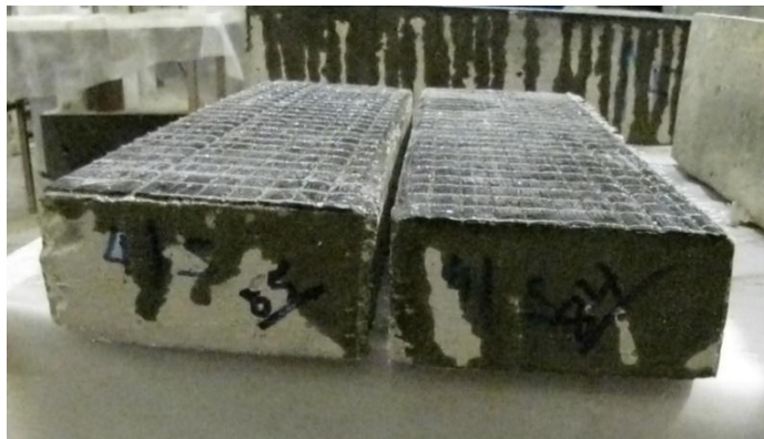
Figure 5.3.5 – Pull-off test samples using FRP wrap
