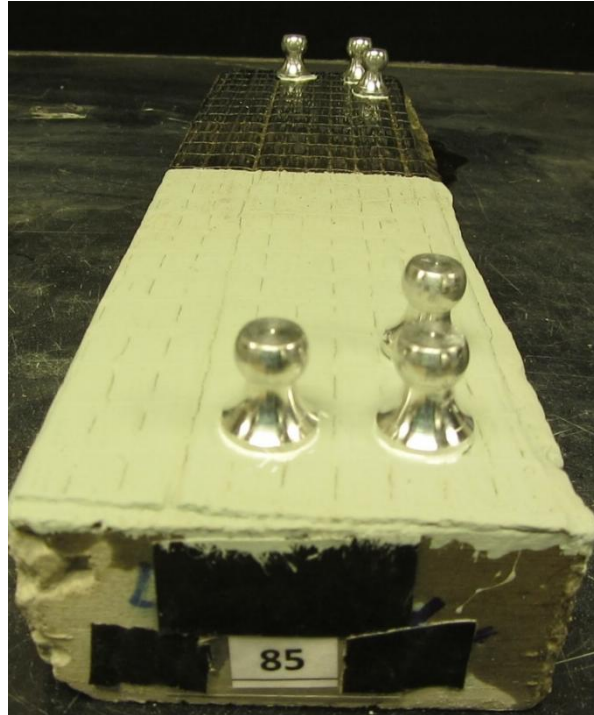
Figure 5.3.11 – Installation of dollies on a half-painted sample
