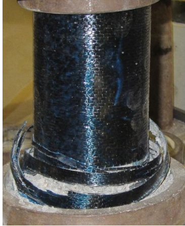
Figure 5.4.10 – Confinement sample 121 FRP failure due to lack of end confinement at the bottom prompting FRP to unravel upward
