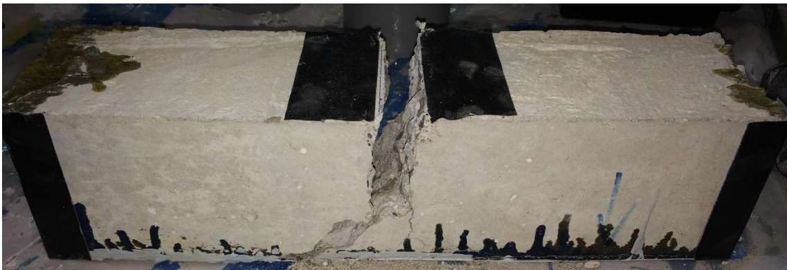
Figure 5.4.4e –Accelerated sample 101 failure plane
