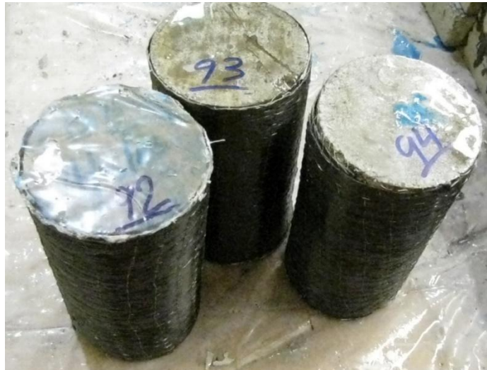
Figure 5.3.6 – FRP strengthened confinement samples
