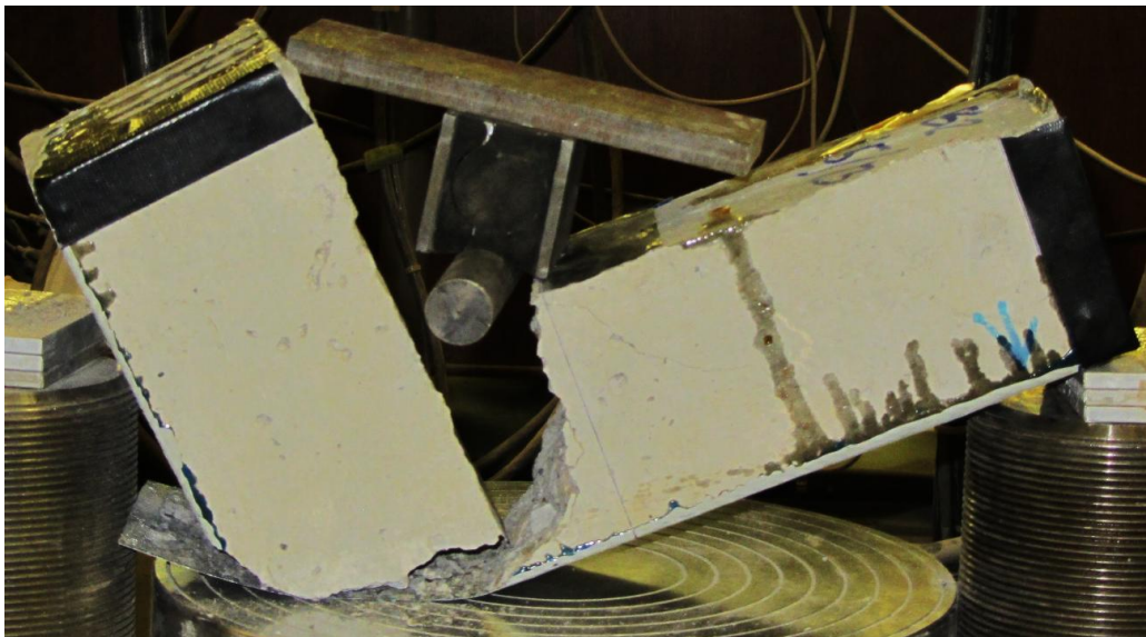
Figure 5.4.6b –Accelerated sample 102 failure (debonding/peeling)
