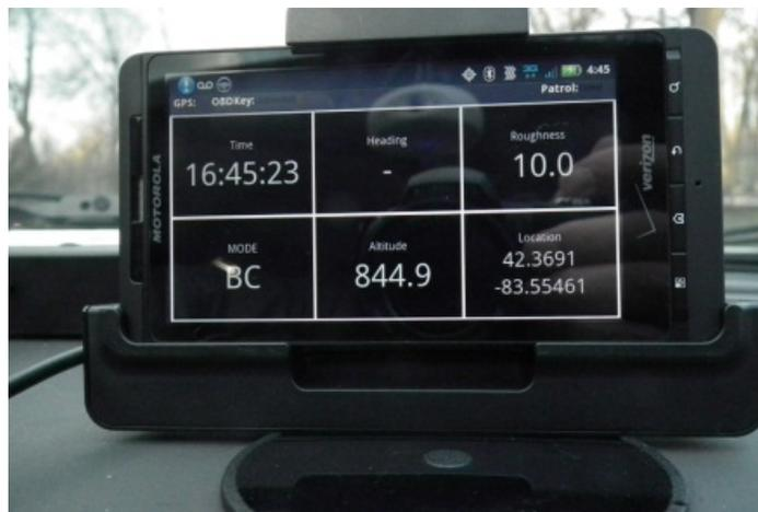
**Figure 3 – The information screen on the Android-based smartphone**
