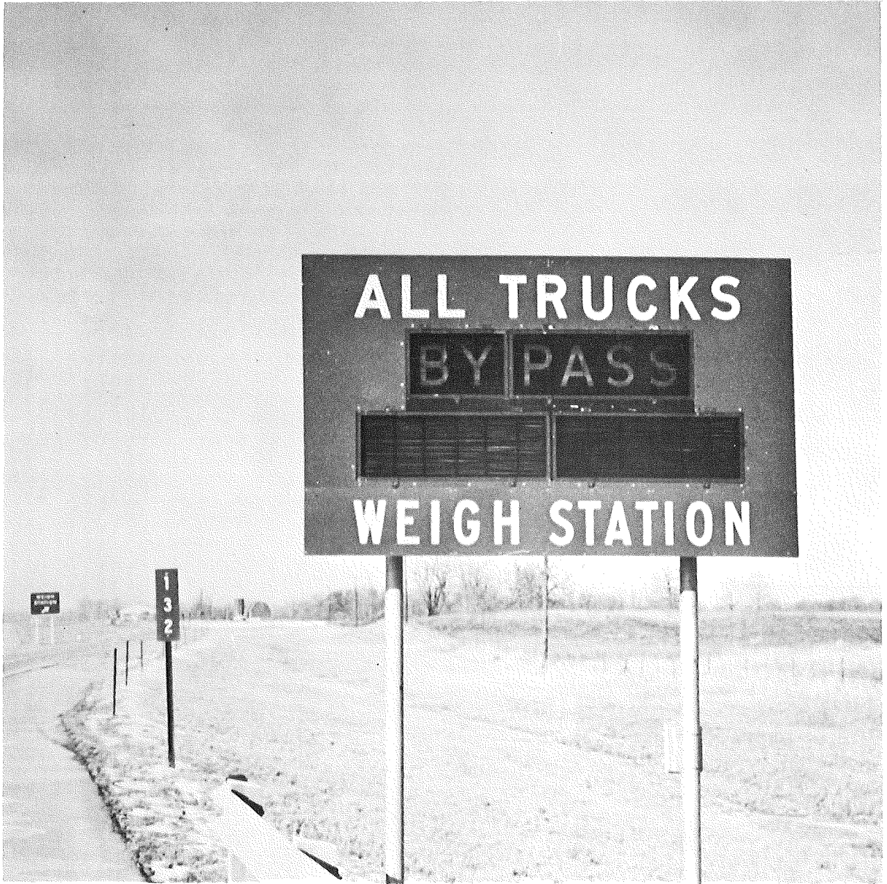
PHOTOGRAPH #3 - FLUORESCENT TYPE SIGN AS USED IN FIELD STUDY
