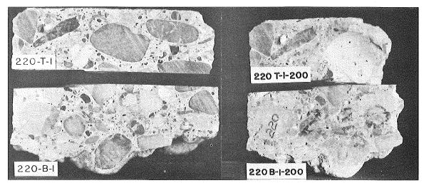
Core No. 220 before and after 200 cycles in water
