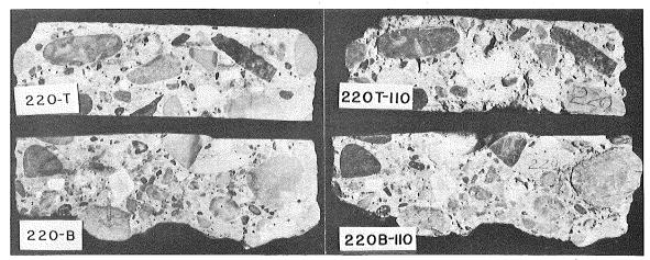
Core No. 220 before and after 110 cycles in 10-percent calcium chloride solution
