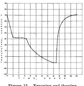
Figure 15. Freezing and thawing temperature cycle.
