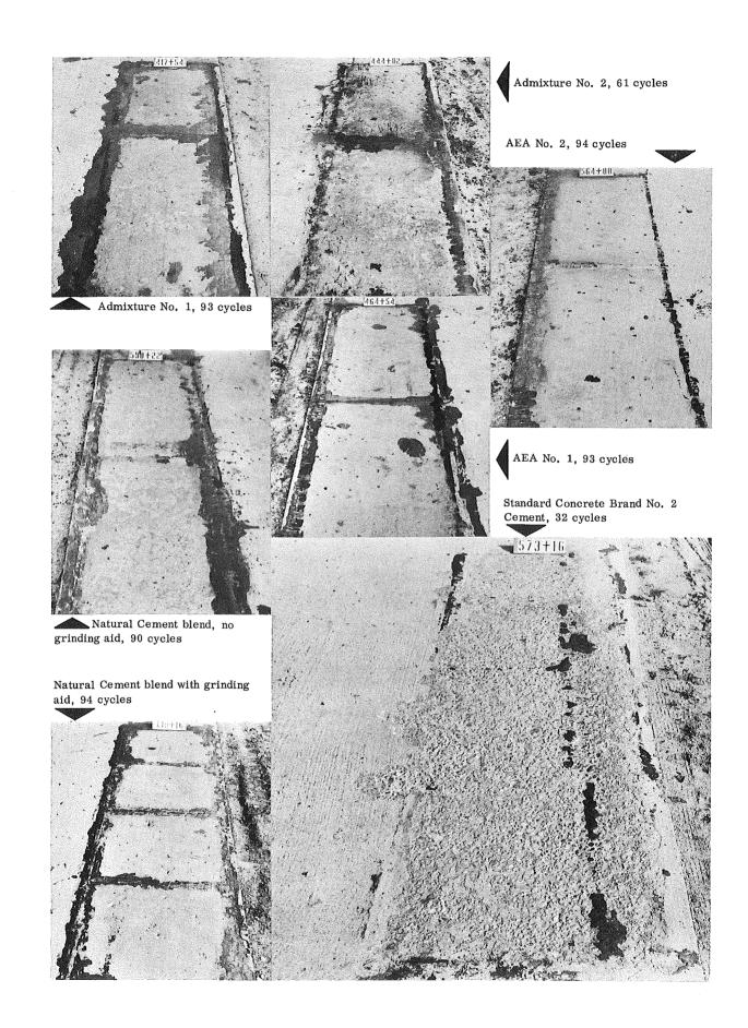
Figure 11. Condition of typical panels at end of accelerated scaling test (continued).
