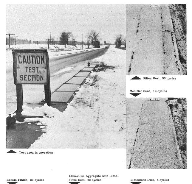
Figure 11. Condition of typical panels at end of accelerated scaling test.
