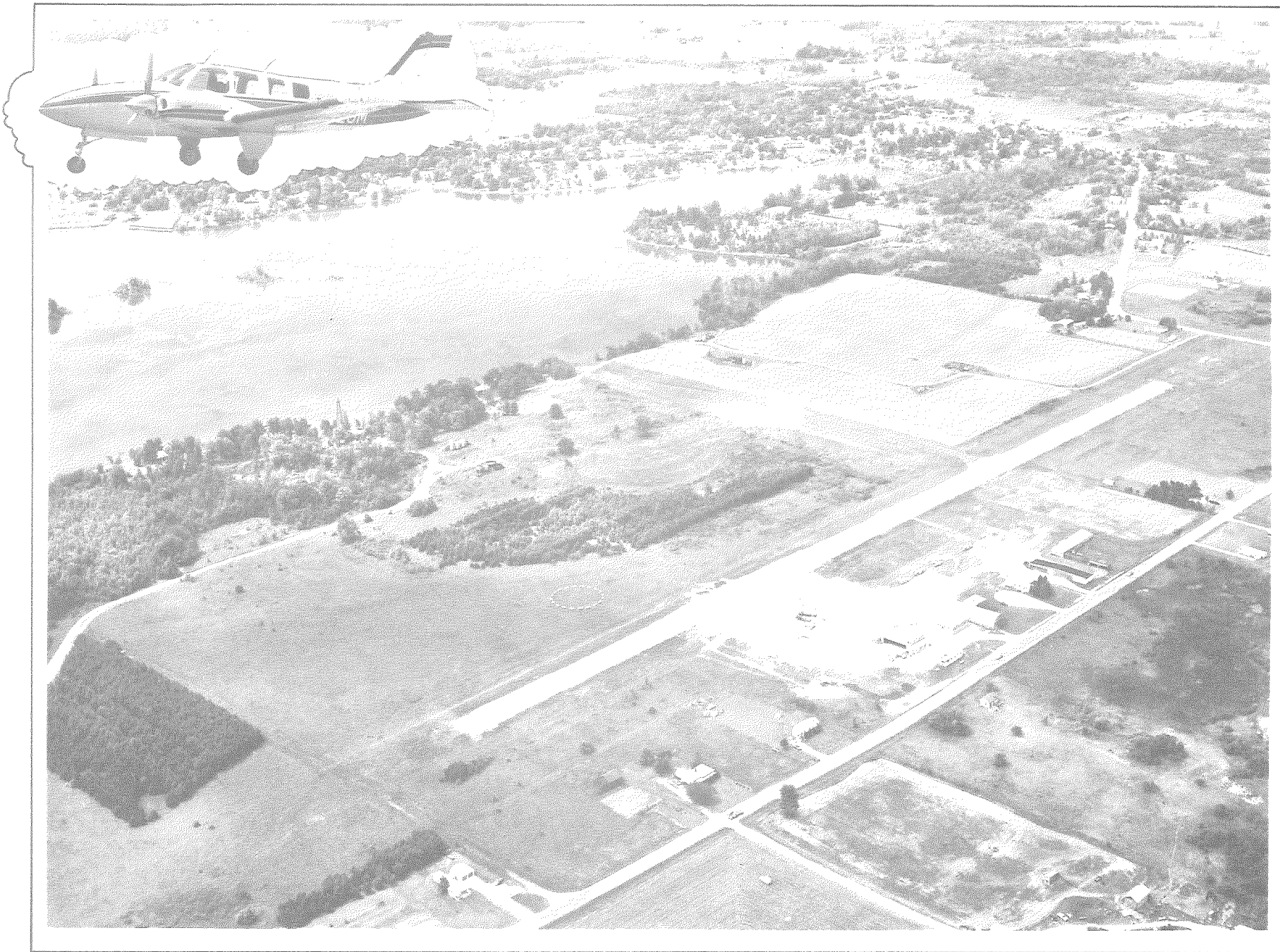
TYPICAL B-II AIRPORT (Basic Utility—Stage II) AIRCRAFT SHOWN, as being typical for this size airport, IS A BEECH BARON
