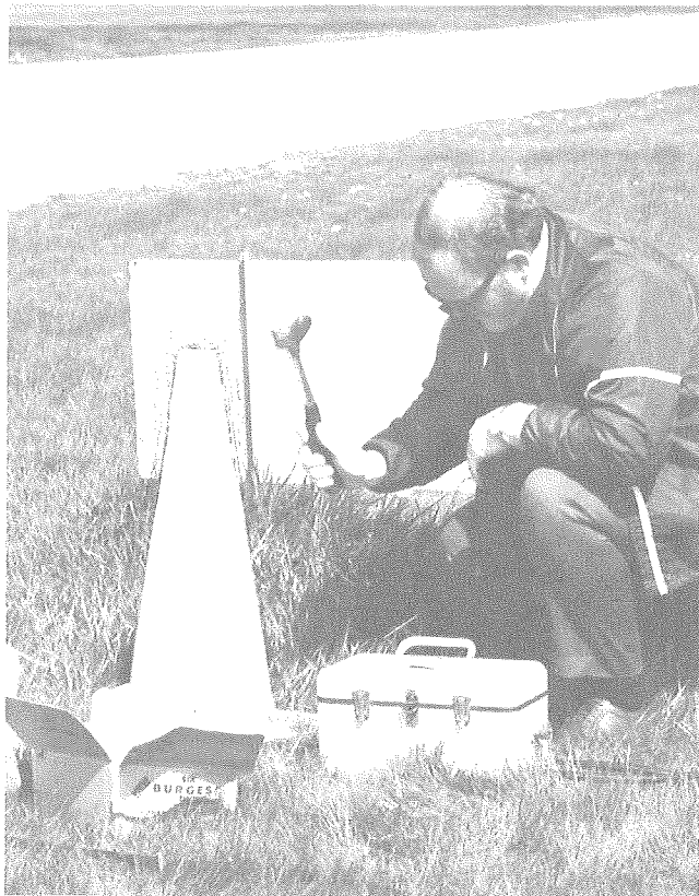
Employee Installing Aircraft Traffic Counter. Impulse Hoses Stretched Across Taxiway
