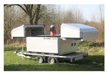
Figure 74: Drone Docking Station Mounted on a Portable Trailer
