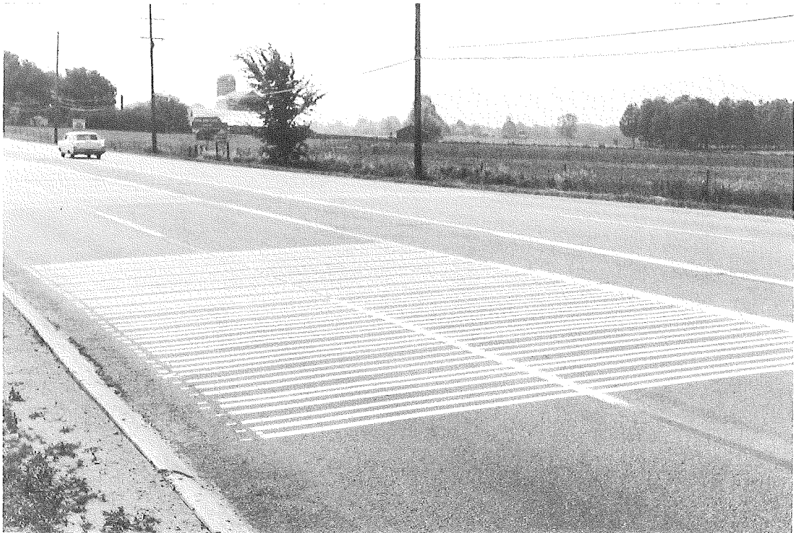
Figure 2. 1959 performance areas shortly after deposition of striping: Area 2, bituminous, in top photo, white and yellow stripes in background adjoining 1958 whites in foreground. Area 4, bituminous, in lower photo with yellow stripes in foreground, and 1958 or older striping in background.
