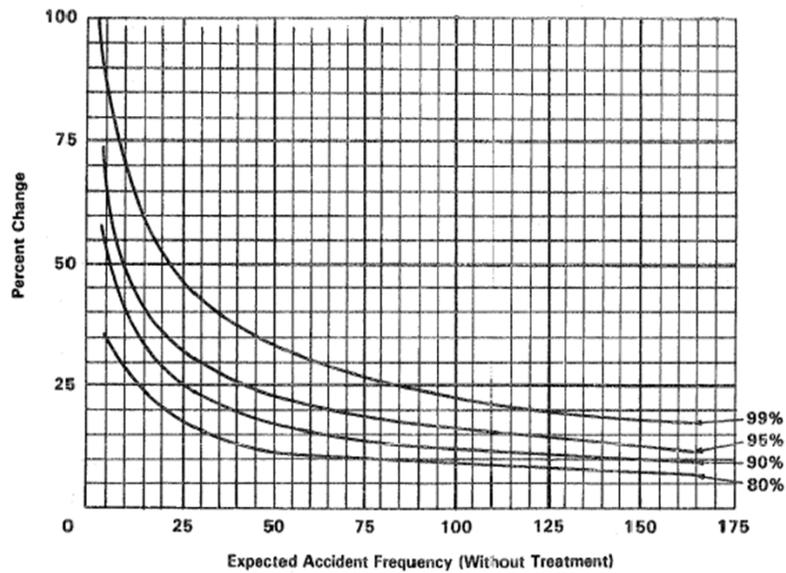
**Figure 7. Poisson Curves for Expected Accident Frequency (13)**
