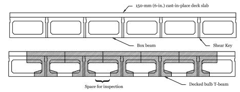
Researchers propose modifying traditional side-by-side box-beam bridge superstructure (top) with decked bulb T-beams (bottom).
