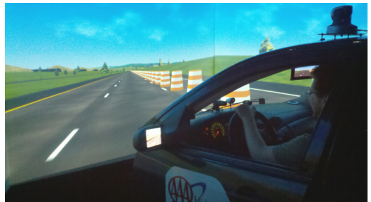
The driving simulator at Central Michigan University’s Center for Driving Evaluation, Education & Research will be used to gather data for the drum spacing project.
