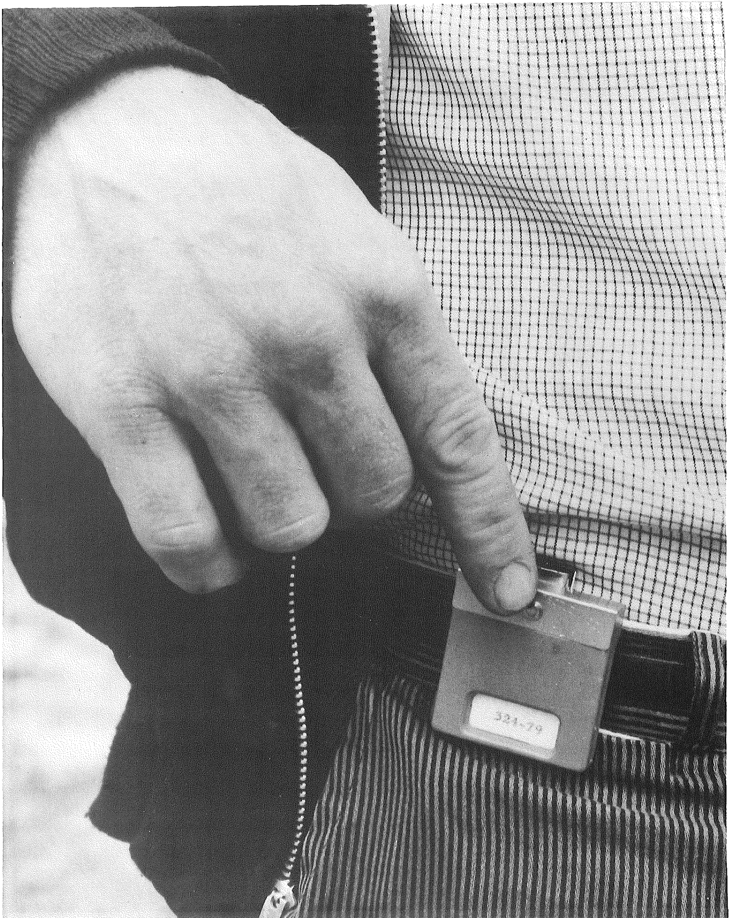
Figure 11. Typical film badge carried by operators using the Michigan Gage.
