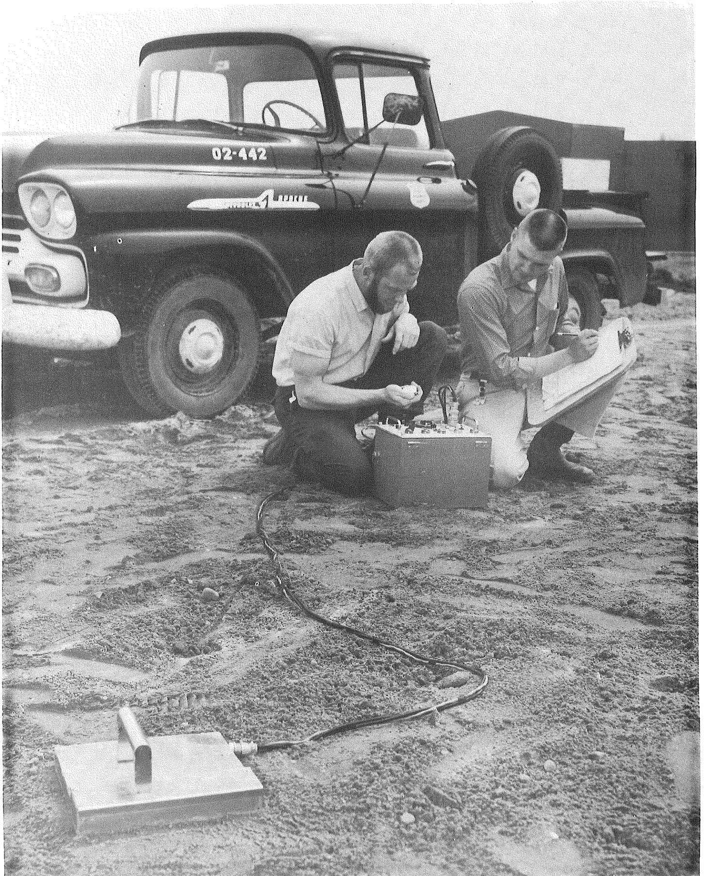
Figure 2. Michigan Gage in use. Operators: Jack Lund and Larry Miller
