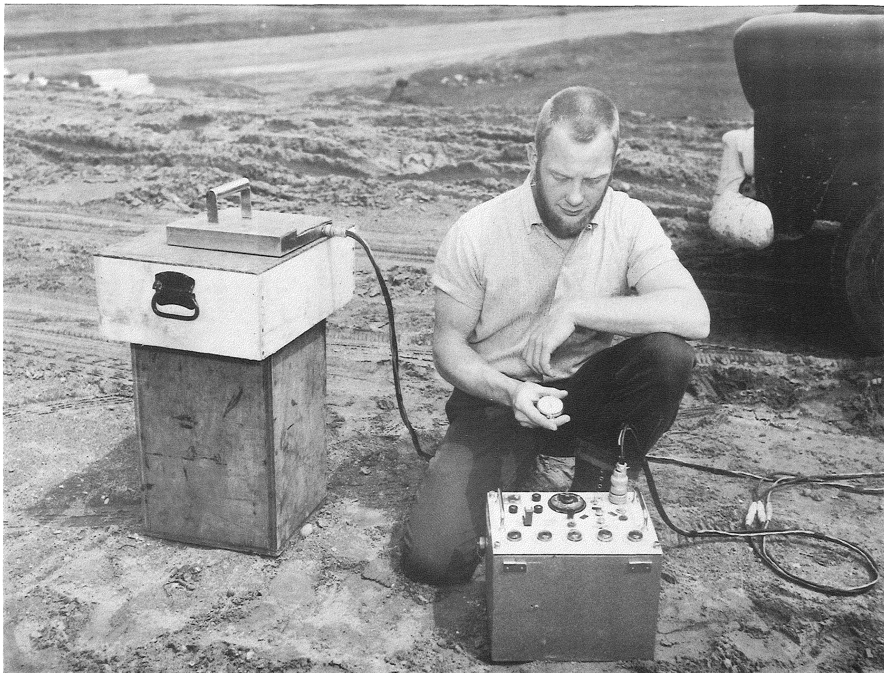
Figure 3. Method of running standard density and moisture count rates with the Michigan Gage. Operator: Jack Lund.
