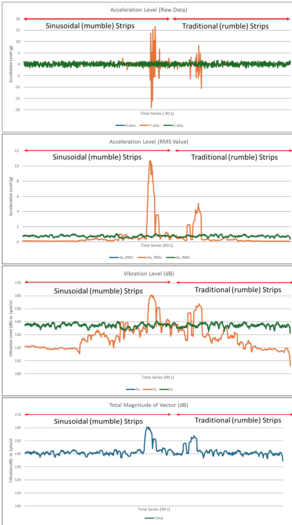
Figure 23. Time-series Data Resulting from Each Step of the Triaxial Acceleration-to-Vibration Data Conversion Process
