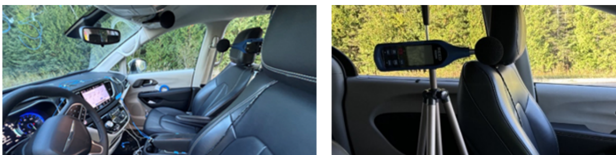
Figure 10. In-Vehicle Noise Measurement Setup
