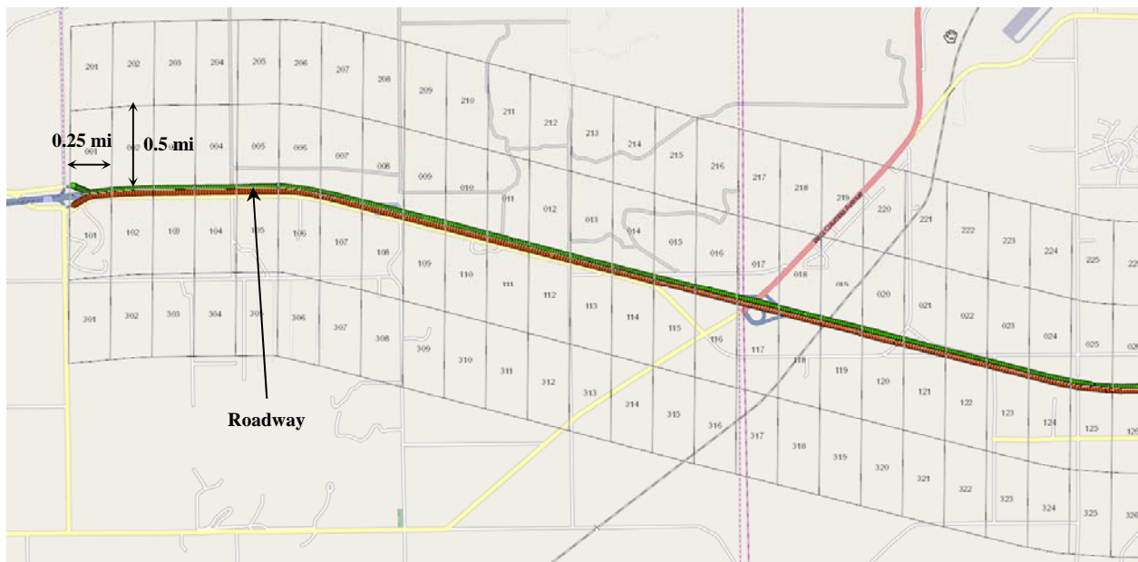
Figure 11. Excerpt of the Grid Created using GIS for Assessment of the Pilot Corridor
