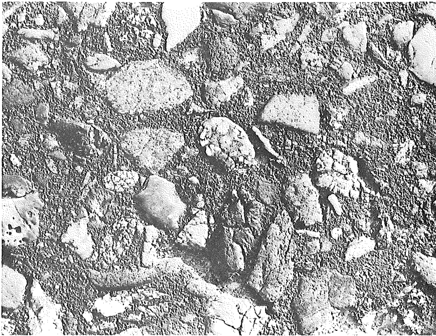
Figure 19—Project 5, Gravel aggregate 26A, Traffic Lane, coef. 0.50. Age 11 years. Average daily traffic, 3920. Wear factor 43.6.
