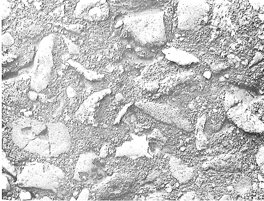
Figure 23—Project 2, Gravel aggregate 25A. Traffic Lane, coef. 0.545. Age 4 years. Average daily traffic, 3120. Wear factor 12.1.
