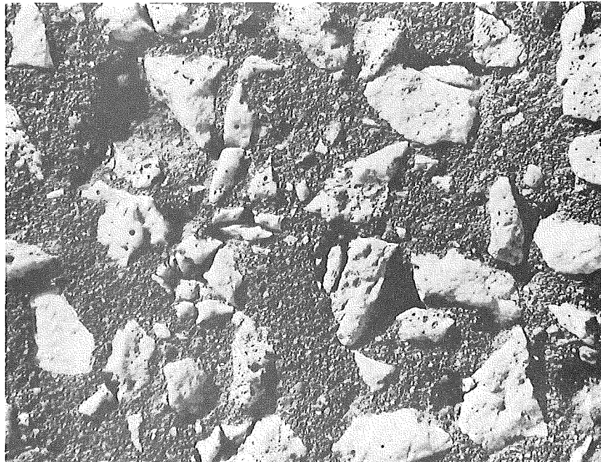
Figure 26—Project 18, Limestone aggregate 25A. Passing Lane, coef. 0.57.
