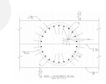
Example Hooked Bar Placement Detail
