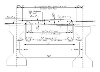
Figure 8: Guide for Reinforcing Slab of Bridge with Prestressed Concrete Beams
