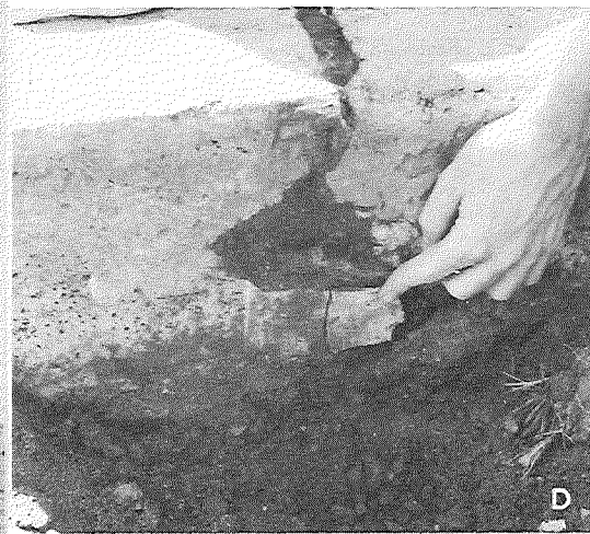
Figure 11. Spalls were observed near the inner edge, near the centerline, and at the outer edge of this joint (A, view from outer edge). Excavation at the outer edge showed fair alignment of the base plate and joint groove (B), with considerable infiltration of foreign material (C). However, excavation at the inner edge (D) showed base plate embedment in the slab concrete. The extreme tilt of the base plate (E) suggests that it may have been moved by paving equipment during pouring or placed on an unlevel base. In either case, the dowel bar assembly may also have been tilted, a possible explanation for the surface spalling. 1392+42; EB; 34044, C1
