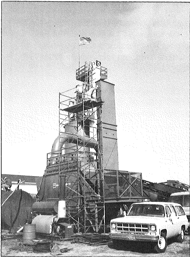
Figure 2. Stack samples (above) being taken at the Hicks asphalt plant (left) near Alma.
