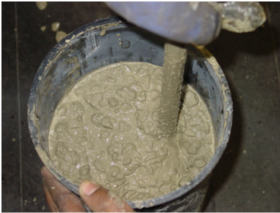
(c) Compaction of concrete cylinders
