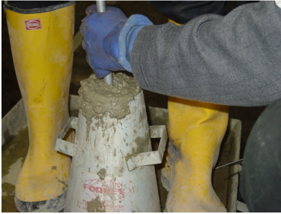
(a) Compaction of concrete during slump test
