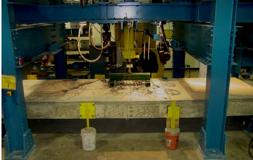
Figure 3.5-4 Load setup (experimental model).
