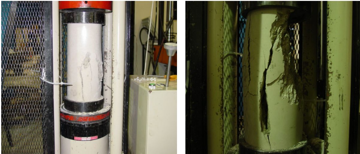
(a) Concrete cylinder being tested
