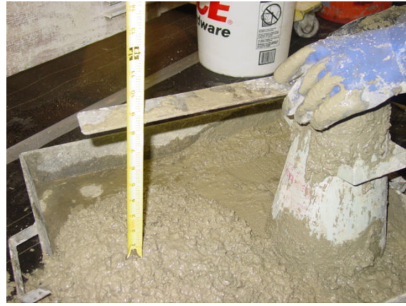
(b) Measuring of concrete slump
