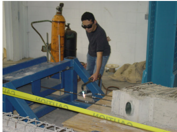
(f) Cutting of pre-tensioning steel strands
