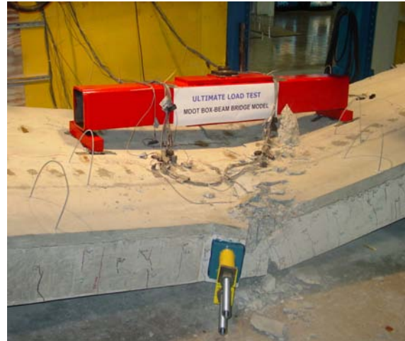
(b) Crushing of concrete
