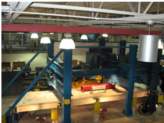
Figure 5.3-20 Experimental setup and instrumentation of the bridge model.
