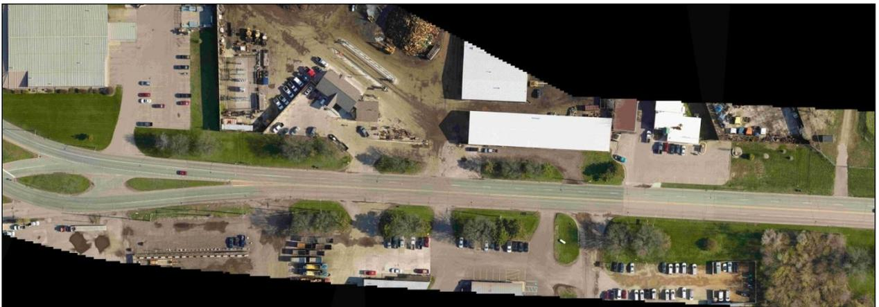
AeroMetric collected asset inventories on seventeen MDOT highway assets. Point assets include catch basins/drop inlets, crash attenuators, delineators, signs, sweepable approaches, and traffic signals. Linear assets include curbs, ditches, guardrail, concrete lane miles, bituminous lane miles, ROW fencing, and shoulders. Lastly, MDOT requested data on mowable acres.
