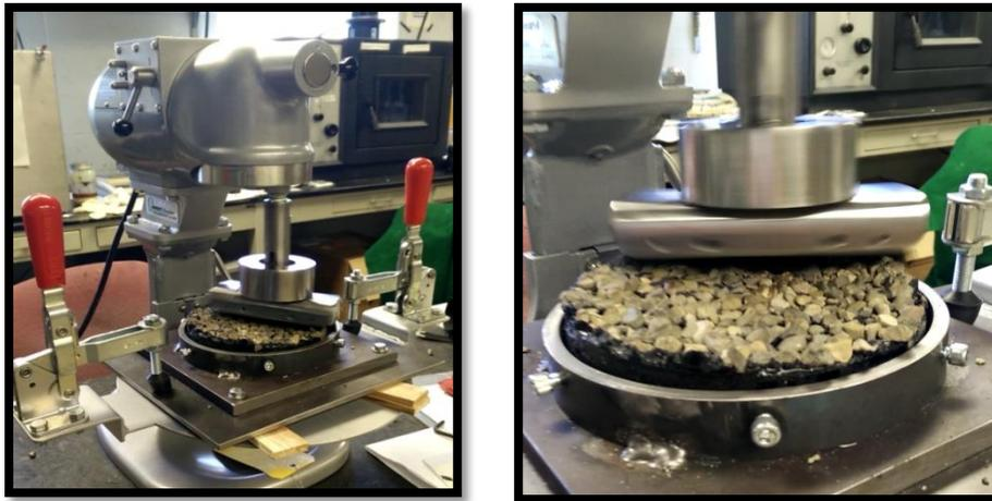
**Figure 30 ASTM D7000 sweep test setup used in the current study**
