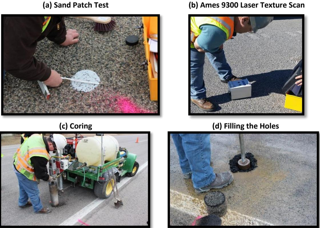
**Figure 6 Procedure for taking cores from the field**
