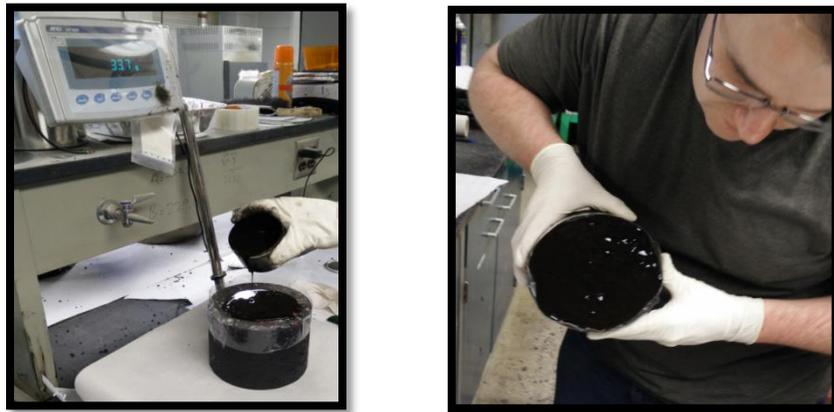
**Figure 10 Binder application process: (a) pouring emulsion on the sample, and (b) spreading the binder by gravity & rotation**
