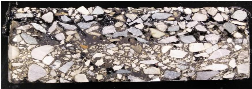
**Figure 31** Cross sectional image of a double chip seal sampled in this study
