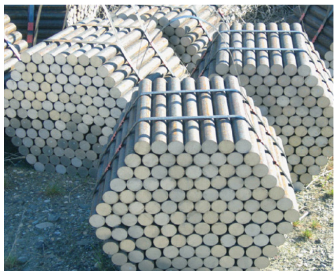
The specialty steel studied in this research is highly resistant to corrosion, making it an excellent building material for bridges and other highway structures.
