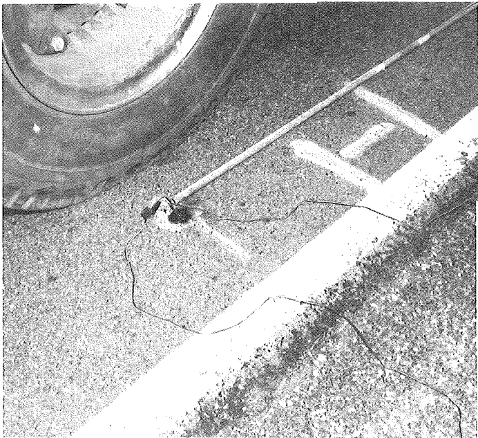
Figure 3. Benkelman beam deflection testing.
