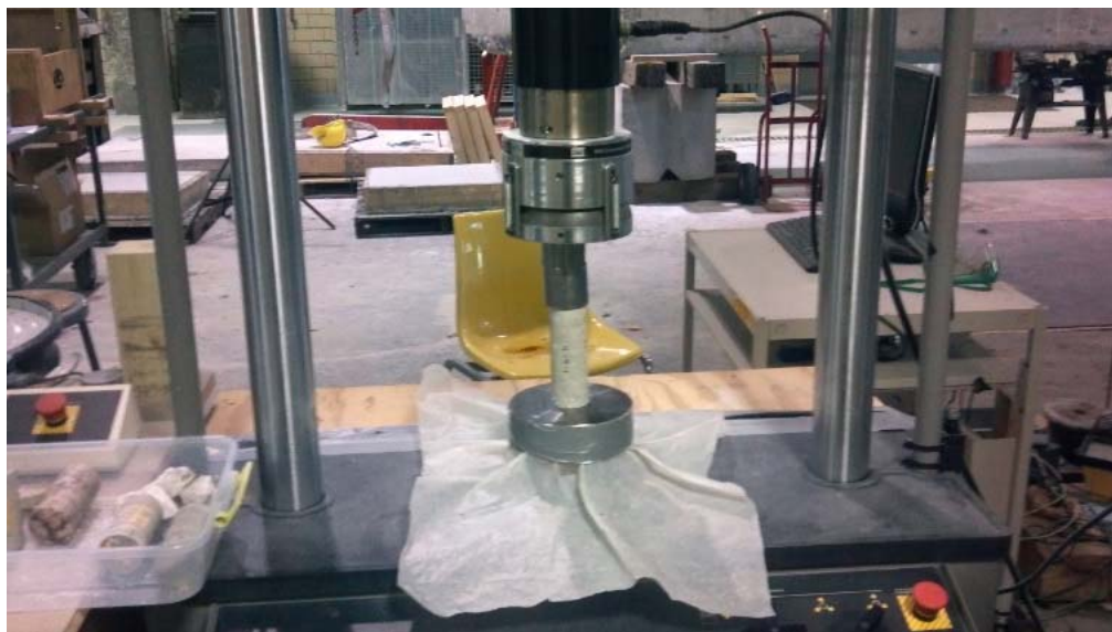
Figure 7: Uniaxial compression testing.
