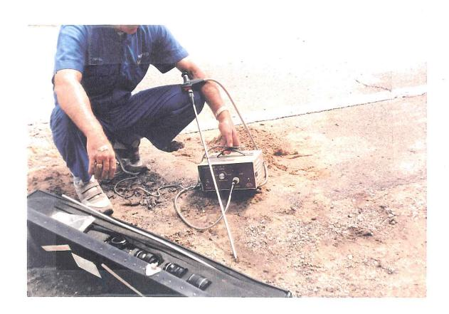
Borescope and power source used in the inspection of the Prefabricated Drainage Systems (PDS)
