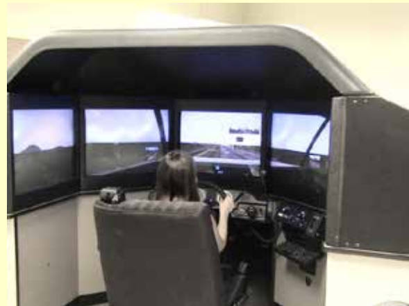
Photograph ES-3. Sample Driver Using the Driving Simulator
