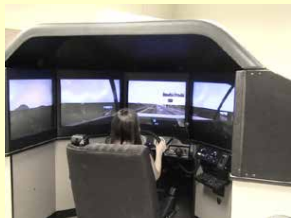
Photograph 4.5. Sample Driver Using the Driving Simulator
