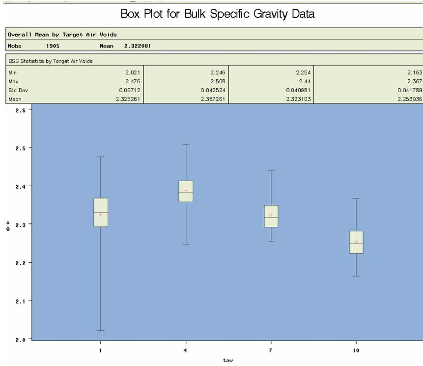
**Figure 4.3 Box Plot of All Bulk Specific Gravity Values by Target Air Void Level**
