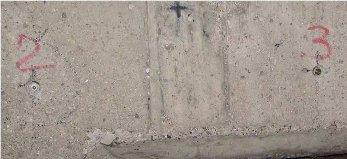
**Figure 4-3 Measuring points with contact seats screwed on brass cylinders**
