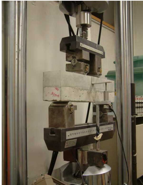
Figure 5.14: Experimental set-up of layered repair system under four-point bending load
