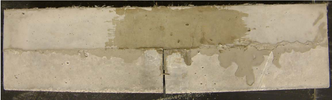
(b) HES-ECC / Concrete (Rough Interface)
