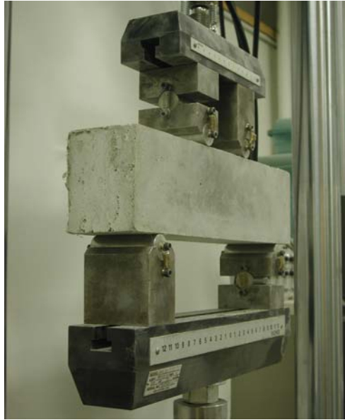
Figure 4.12: Third-point bending test setup
