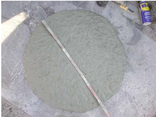
Figure 9.11: HES-ECC show self-compacting property (Flowability test slump diameter = 25.6")
