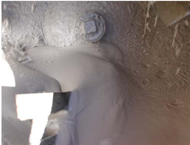
b) After adding sand, water, HRWR and hydration stabilizer
