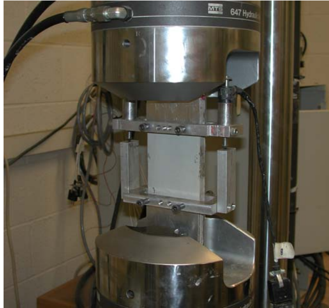
Figure 4.2: Uniaxial tensile test setup
