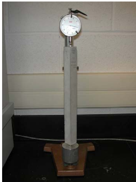
Figure 4.15: Free drying shrinkage test setup
