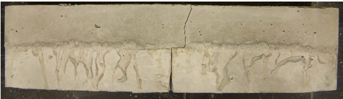
(c) HES-Concrete / Concrete (Smooth Interface)
