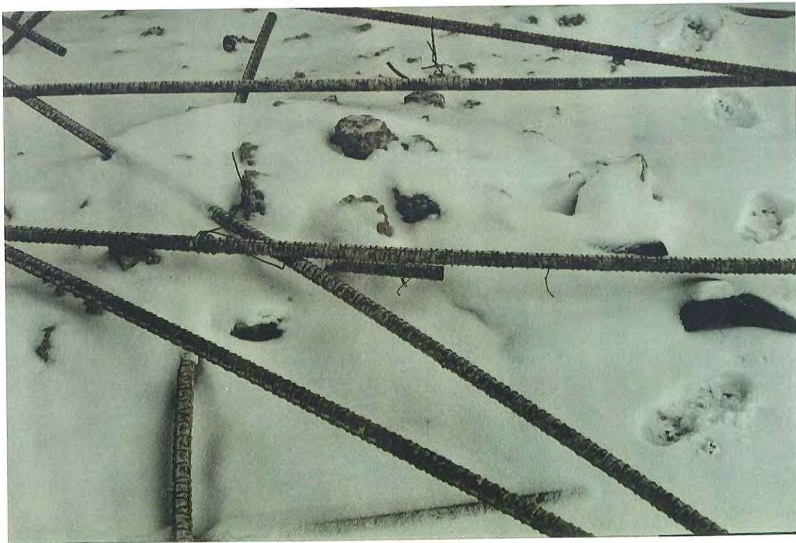
Figure 7. Reinforcing steel presumably taken from Pier 40 during demolition. Note that very little corrosion has taken place; the rust visible on the surface of the bars could have been present at construction or could have occurred after demolition.
