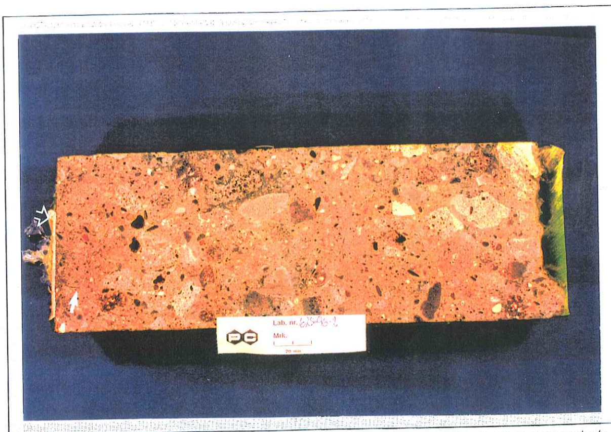
Photo 2. Macrofoto of sample 625-96-2. At surface grey epoxy layer is present. The layer do not penetrate the concrete. Surface crack is present, see arrow.
