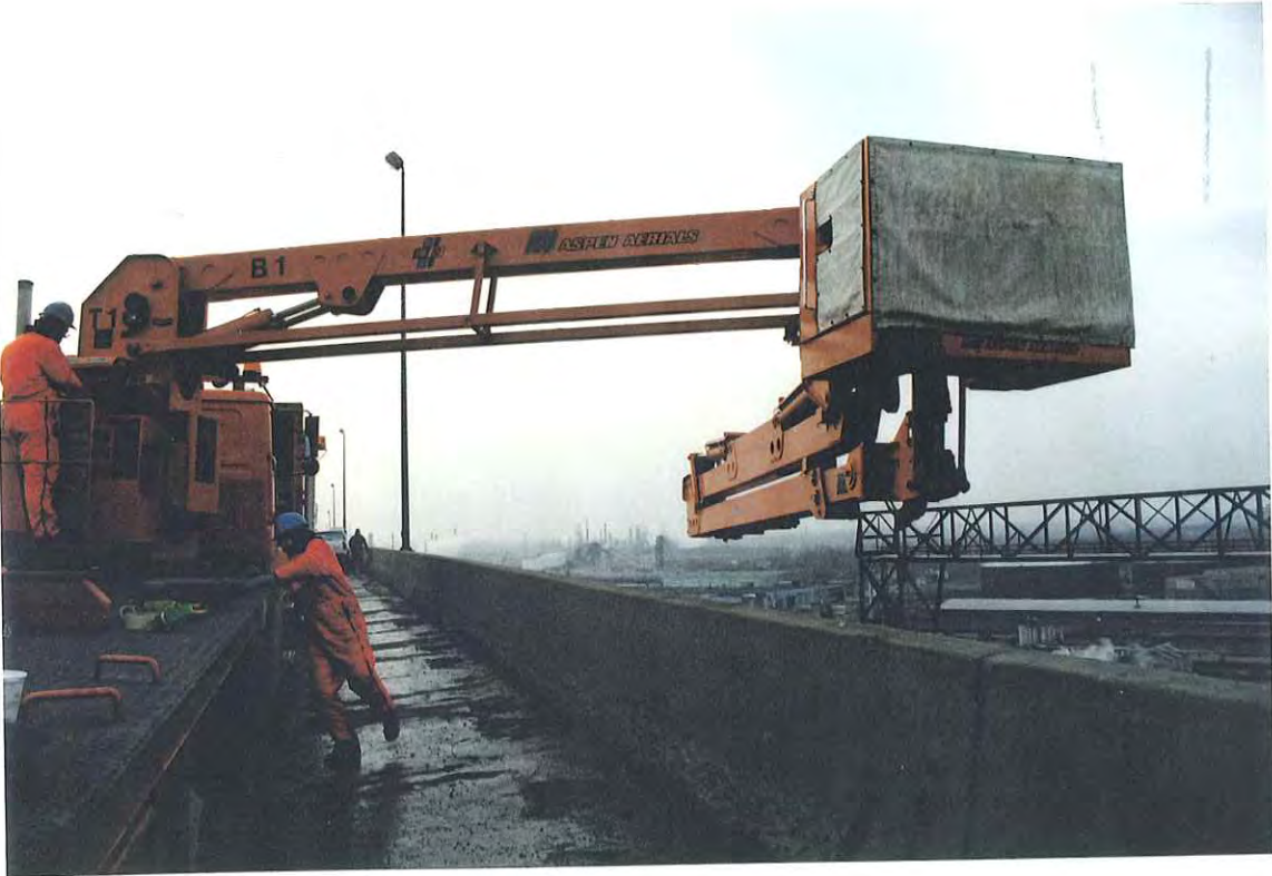
Figure 3. A reach-all provided access to the bridge piers for observation and coring.
