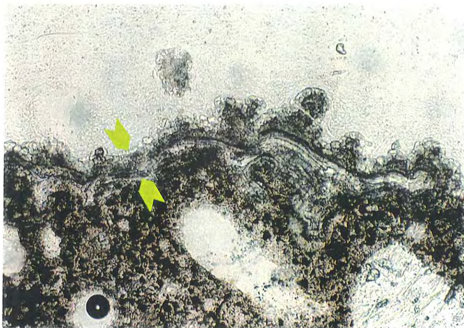
Figure 17. Thin section photomicrograph of core #2 from Pier 38 north face, north-bound, showing inter-layered alkali-silica gel and calcium carbonate deposits (between arrows) on crack wall. Plane-polarized light. Width of field is approximately 350 \mu m.
