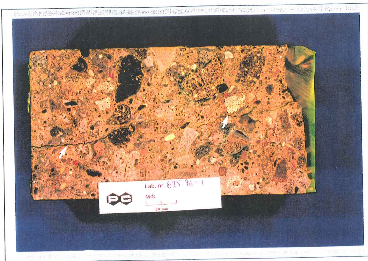
Photo 1. Macrofoto of sample 625-96-1. The concrete contains homogenous distributed slag particles in Portland cement paste. A macro crack penetrates the core perpendicular to surface.
