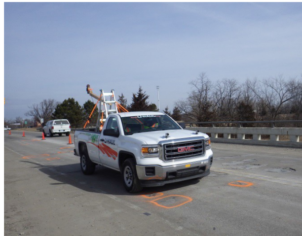
Figure 13: 3DOBS and BVRCS data collection was conducted in unison as the vehicle drove each lane of the bridge.
