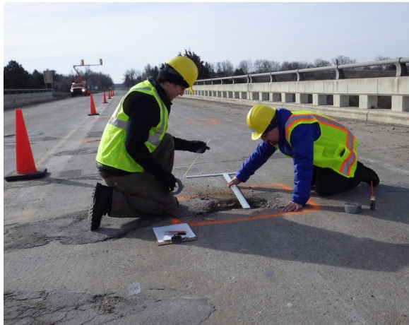
Figure 12: Manual measurements the length, width, and depth of spall and patch features on the bridge deck.
