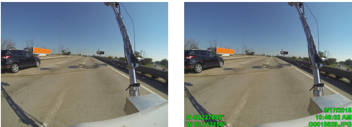
Figure 9: Image collected by the GoPro Hero3 camera (left) and the GeoJot+ processed geotagged image (right).
