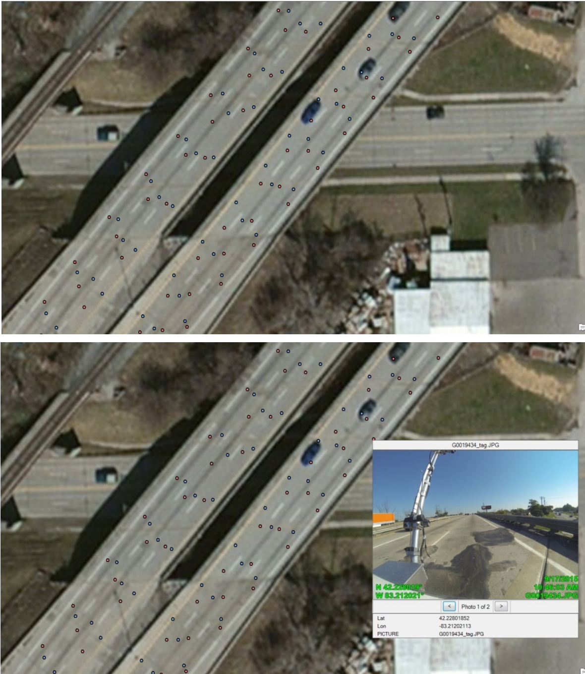
Figure 20: A subset of the I-75 NB/SB Bridges with BVRCS GPS data placed on the bridge (top) and the image showing the bridge deck section that corresponds to the GPS data point (bottom).
