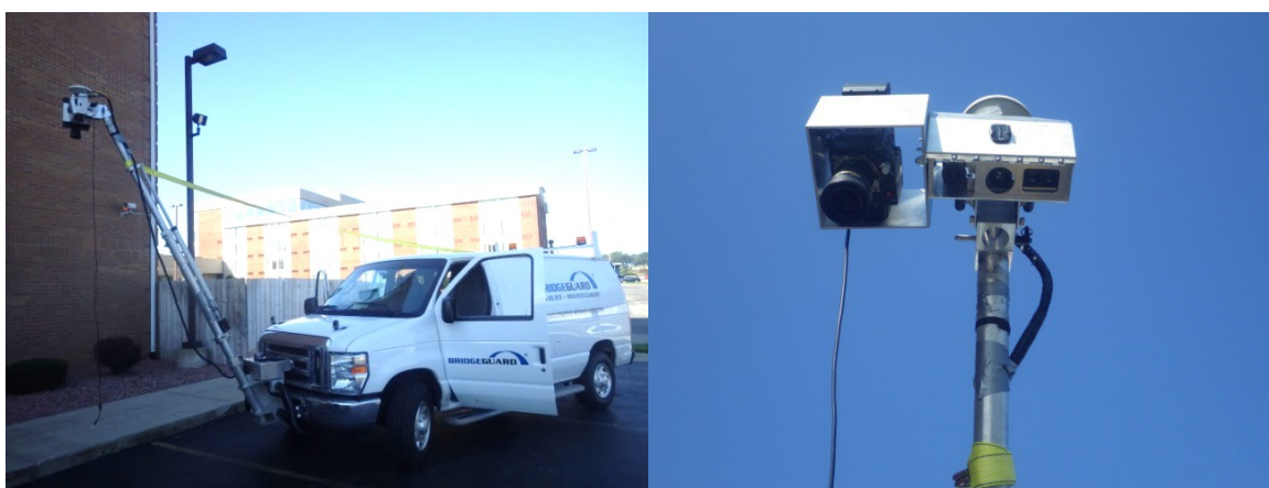
Figure 22: The data collection vehicle (left) and both the RED Epic and FLIR thermal infrared cameras attached to the vehicle.
