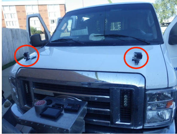
Figure 8: The two GoPro Hero 3 cameras set up on the data collection vehicle hood.
