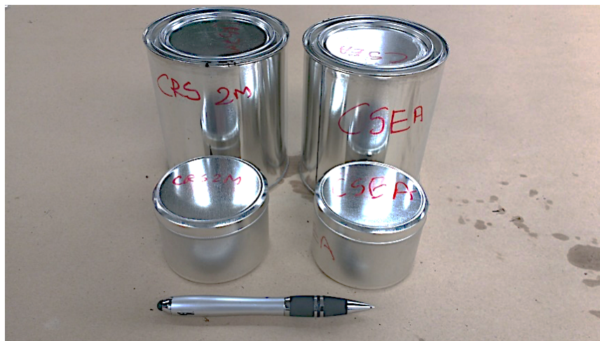
Figure 4-5 Image showing emulsions split and stored into small containers for further testing.
