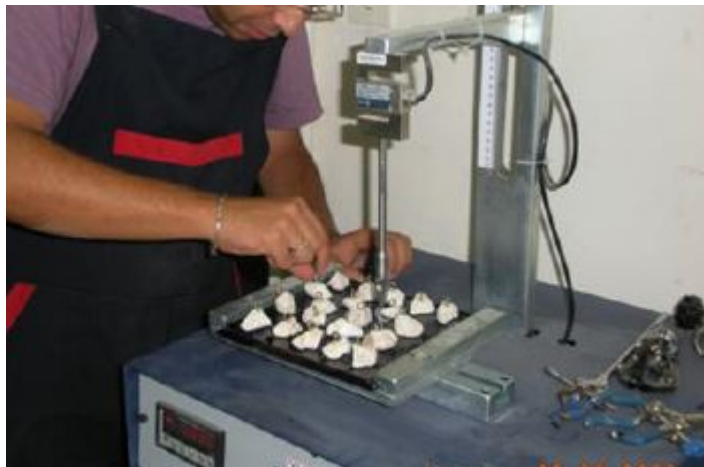
Figure 2-3 Aggregate pullout test setup (source: Akýllý et al. 2012)
