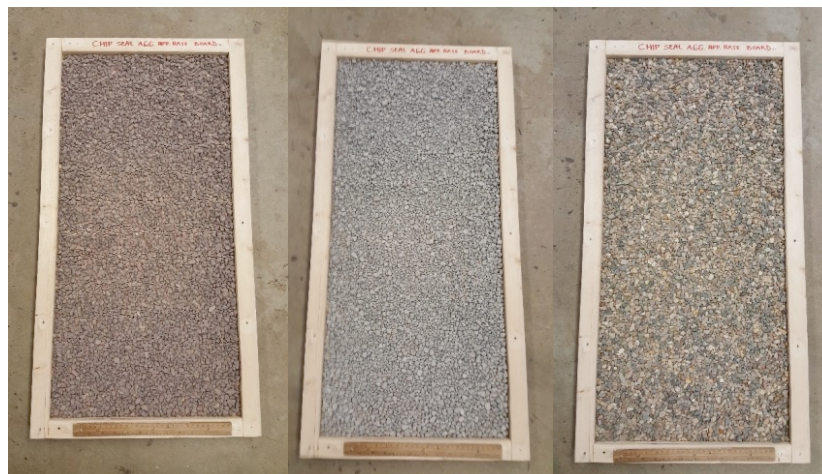
Figure 5-13 Board Test for determining design AAR for natural, slag, and Gerkin aggregates (left to right).
