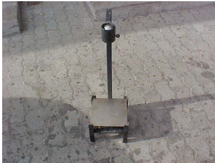
Figure 2-1 Vialit test setup (source: Louw et al. 2004)
