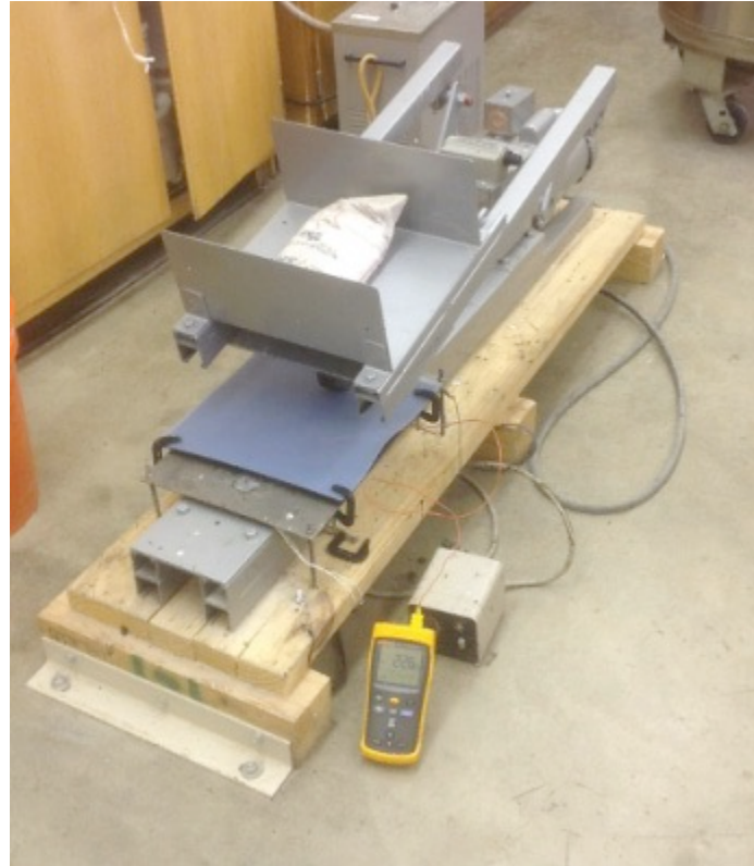
Figure 2-8 Loaded wheel test (LWT) setup (source: Chaturabong et al. 2015)
