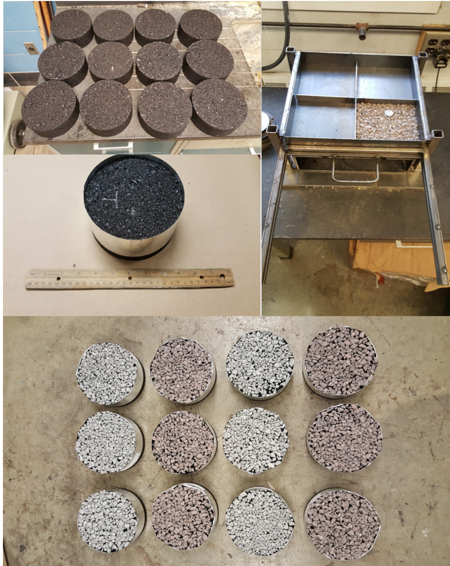
Figure 4-13 Several steps of chip seal specimen fabrication
