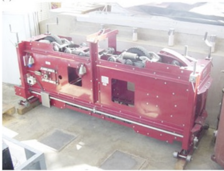
Figure 2-9 MMLS3 setup (source: Adams et al. 2014)
