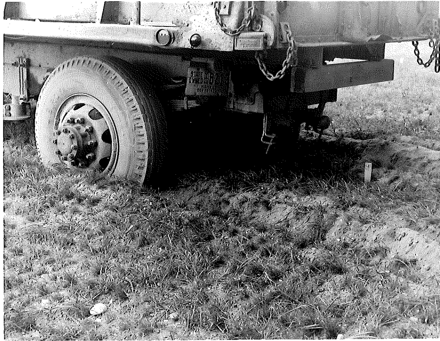
Figure 5. General view showing penetration of truck wheels into dry plots containing graded sand and 10% Miami top soil.
