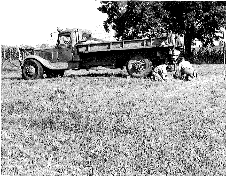
Figure 3. Method of conducting bearing test.
