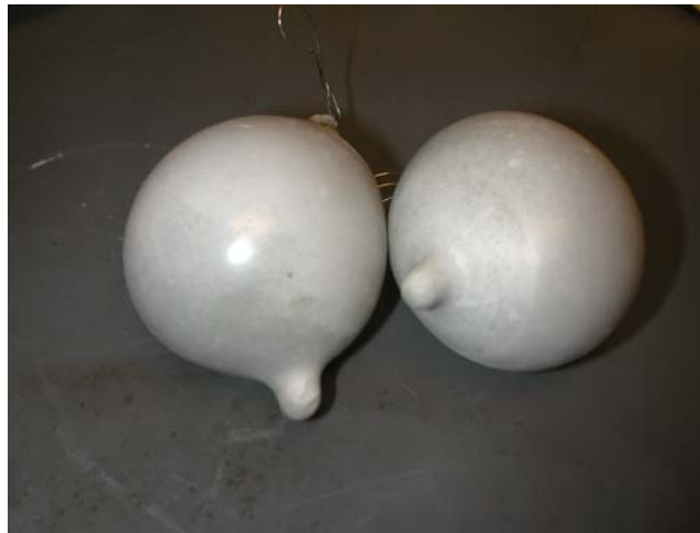
Figure 5.3: Polyurethane membranes with reservoir filled with ECC
