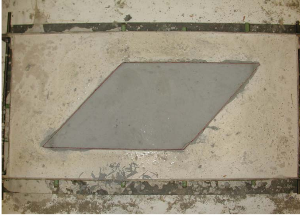
Figure 4.10: Small frame restrained shrinkage test on LS-ECC
