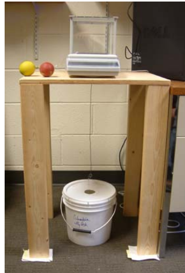
Figure 5.2: Test setup of autogenous shrinkage measurement of ECC
