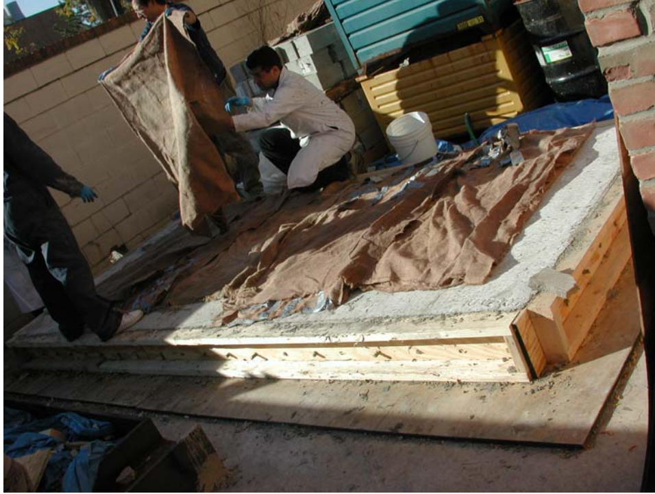
Figure 4.16: Large frame restrained shrinkage test – curing
