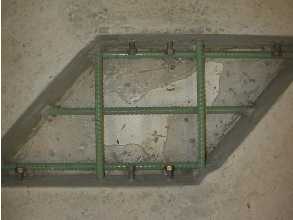
Figure 4.9: Restrained small frame test setup with consideration of skew angle and the presence of steel rebars as stress concentrators
