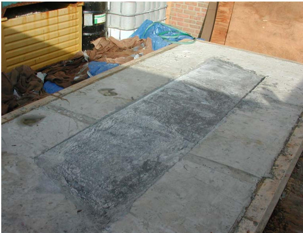
Figure 4.17: Large frame restrained shrinkage test
