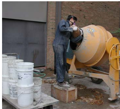
Figure 1.6: The gravity-based mixer used for producing large frame restrained shrinkage test of ECC slab
