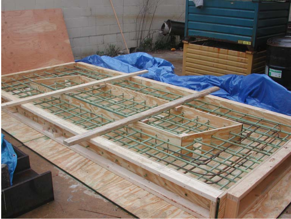
Figure 4.12: Large frame restrained shrinkage test – wood formwork construction
