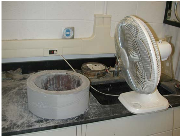
Figure 3.4: Use of 14” fan to provide constant wind effect at early age
