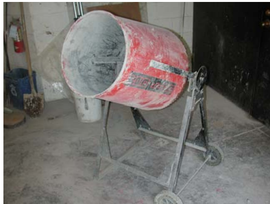
Figure 3.3: A 1 cubic foot capacity gravity mixer
