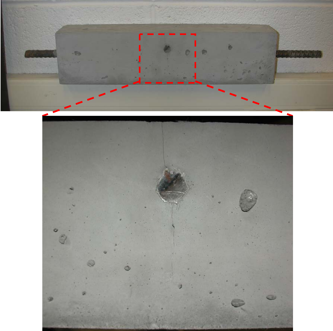
Figure 3.6: A single crack initiated from the transverse rebar
