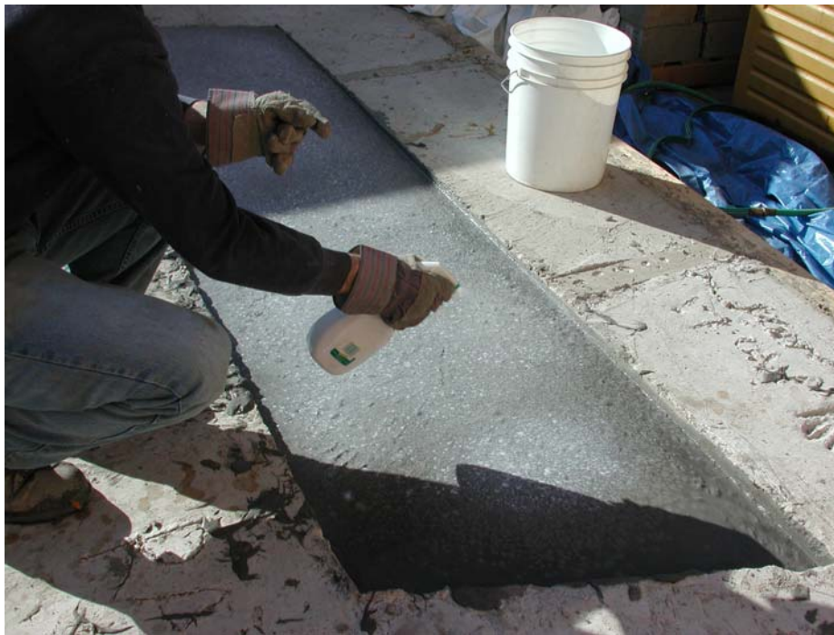
Figure 4.15: Large frame restrained shrinkage test – applying curing compound
