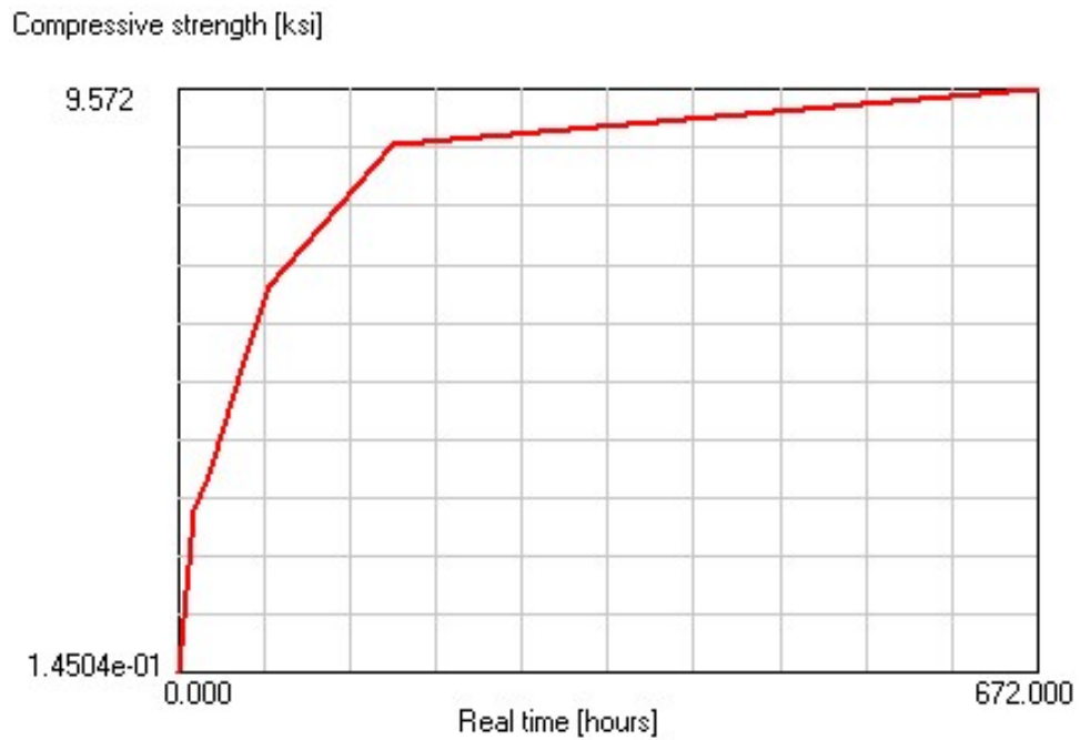
Figure 3.11: Age-dependent compressive strength of ECC
