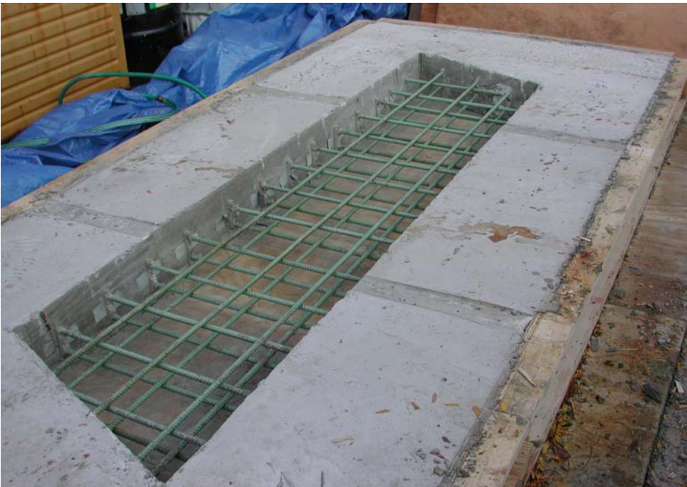
Figure 4.13: Large frame restrained shrinkage test – 20" peripheral concrete frame
