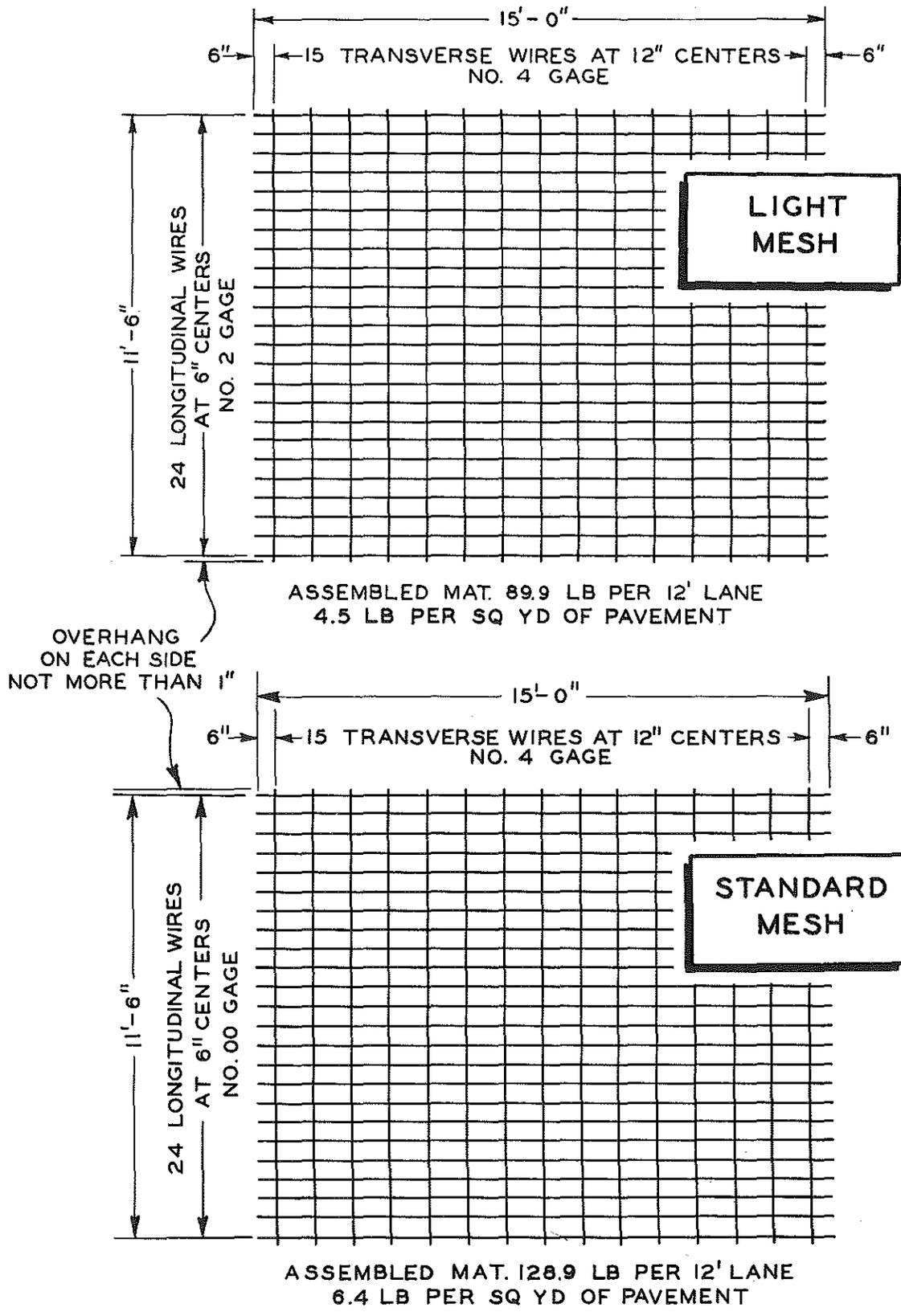
Figure 4. Details of light and standard mesh reinforcement.
