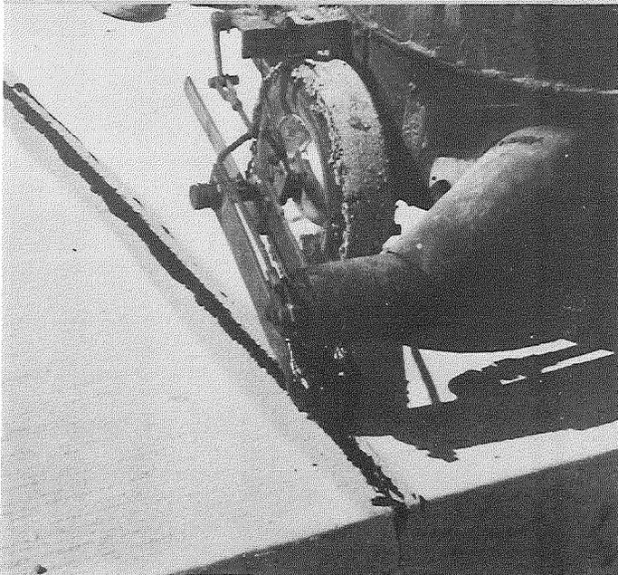
Figure 25. Double-boiler, thermostatically controlled kettle (upper left).
