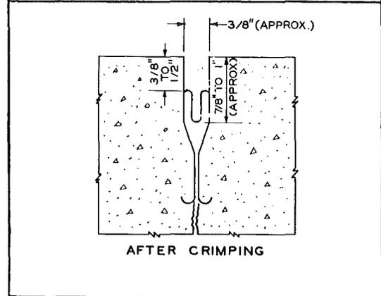
Figure 16. Cross-sections of Unitube joint.
