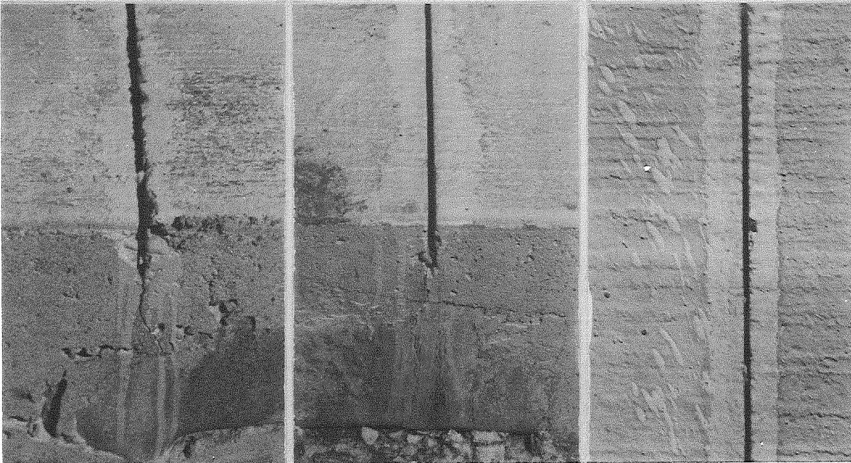
Figure 20. Sawcutting transverse joint grooves with diamond blades is shown above. Typical plane-of-weakness cuts include one at a vibrated joint 6 to 7 hr after pour (lower left), at a vibrated joint 15 to 18 hr after pour (lower center), and at a non-vibrated joint 24 to 25 hr after pour (lower right).
