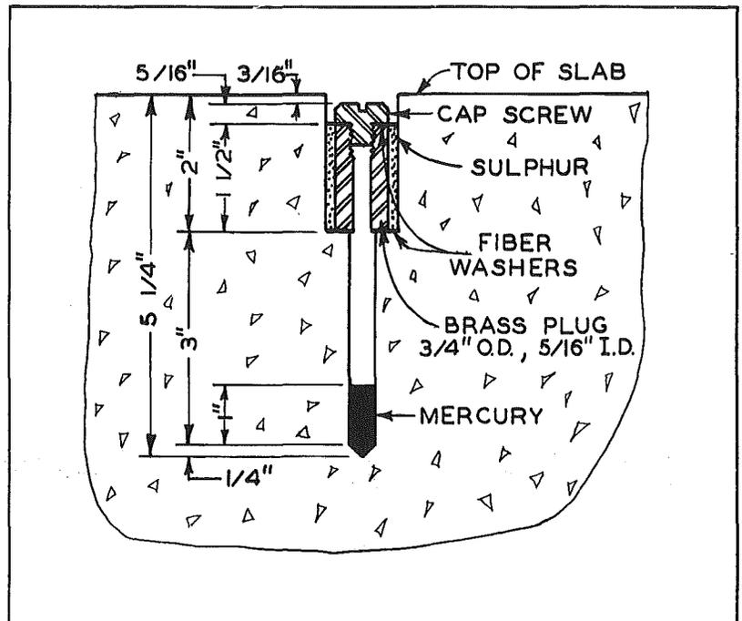
Figure 32. Cross-section of temperature well (above).
