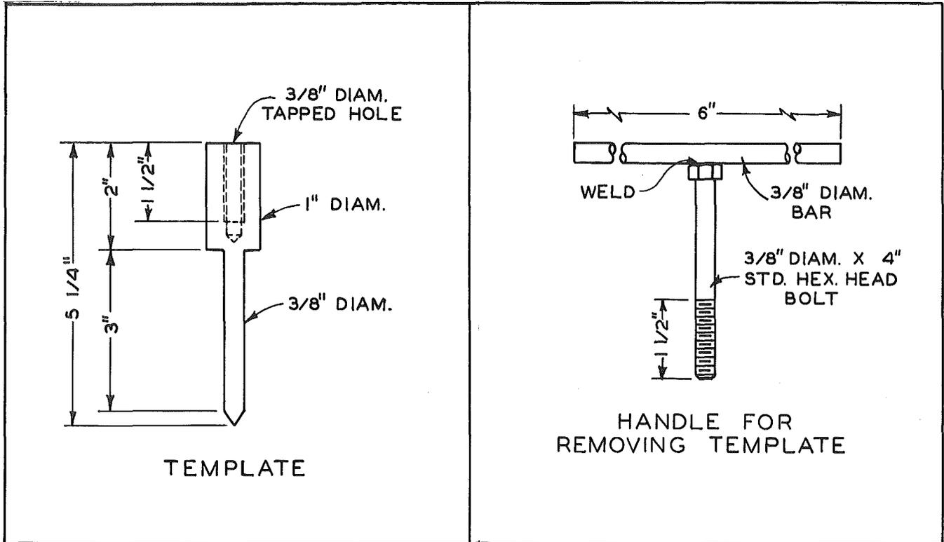
Figure 31. Template for forming temperature well.
