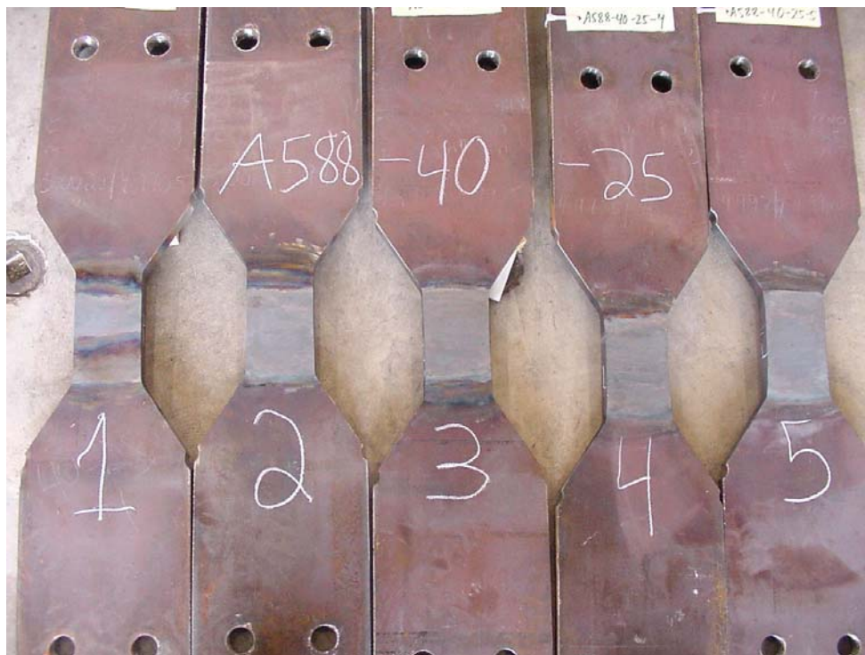
Figure 5.25 Frontal view of A588-40-25 specimens after experimental investigations
