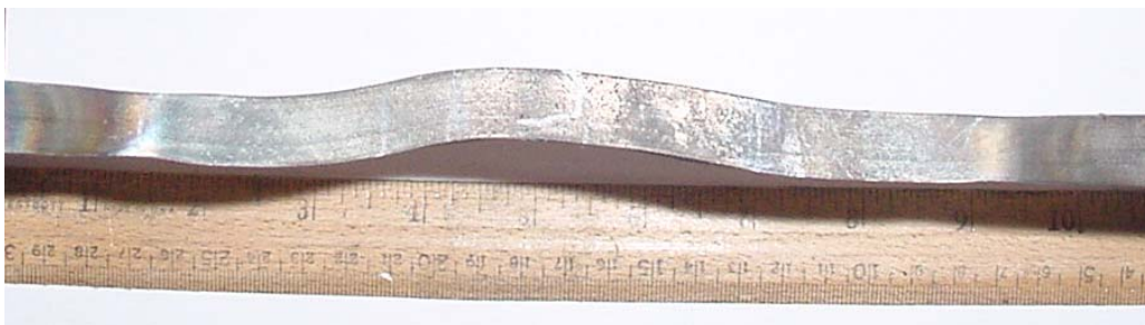
Figure 5.49 Induced curvature in the test area of Specimen A7-90-40-3
