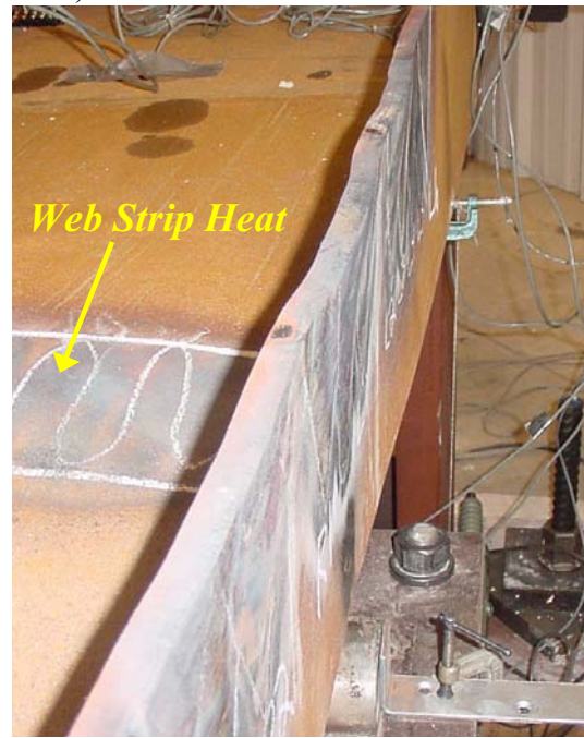
Figure 8.20 Location of strip heats applied to the web of A7-Beam 2
