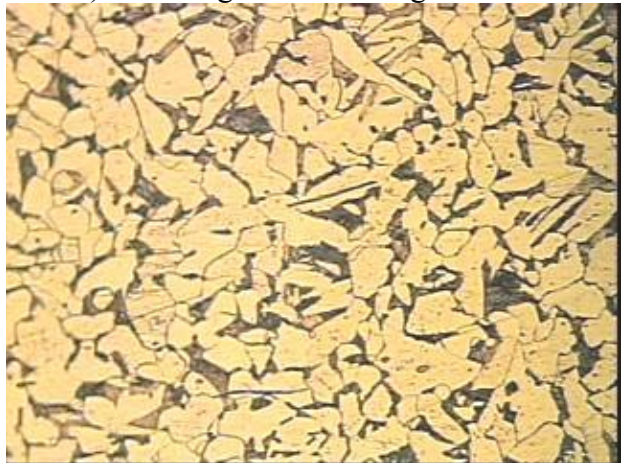
Figure 7.23 Microstructure of undamaged A7, A36, and A588 steel
