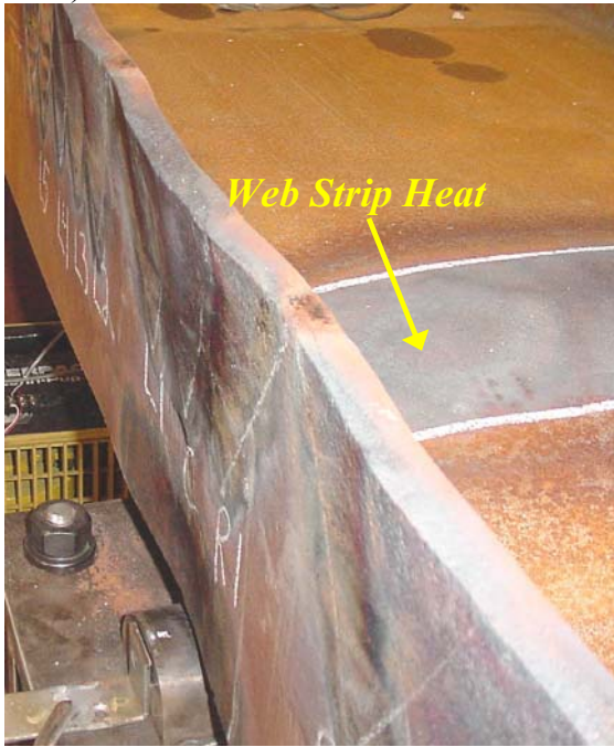
Figure 8.20 Location of strip heats applied to the web of A7-Beam 2
