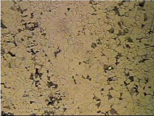
Figure 3.17 Microstructure of heated and unheated portions of the Lansing Road Bridge
