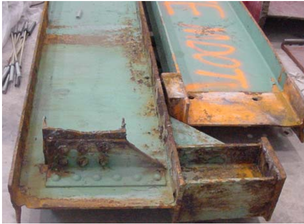
c) Beam used for the fabrication of small scale experimental tests.
