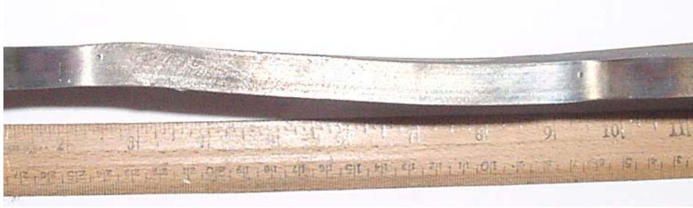
Figure 5.46 Induced curvature in the test area of Specimen A7-90-25-1
