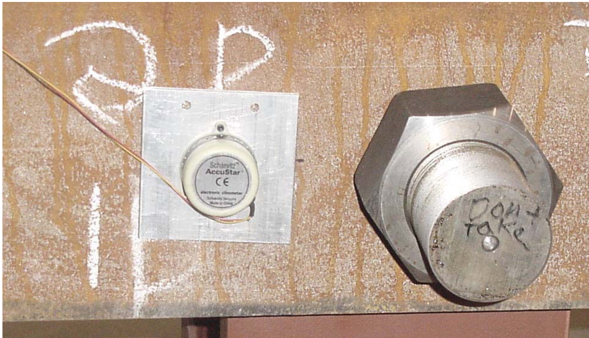
Figure 7.12 Location of rotation meter in respect to roller support
