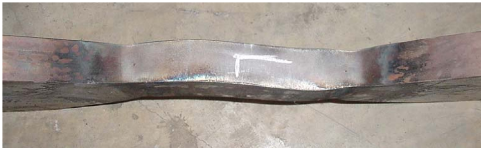
Figure 5.15 Double curvature in the test area of Specimen A36-90-25-5 when complete
