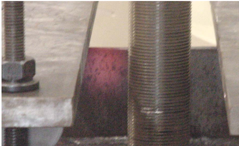
Figure 8.37 Opposite side of Vee heated to a maximum temperature of 1400 °F
