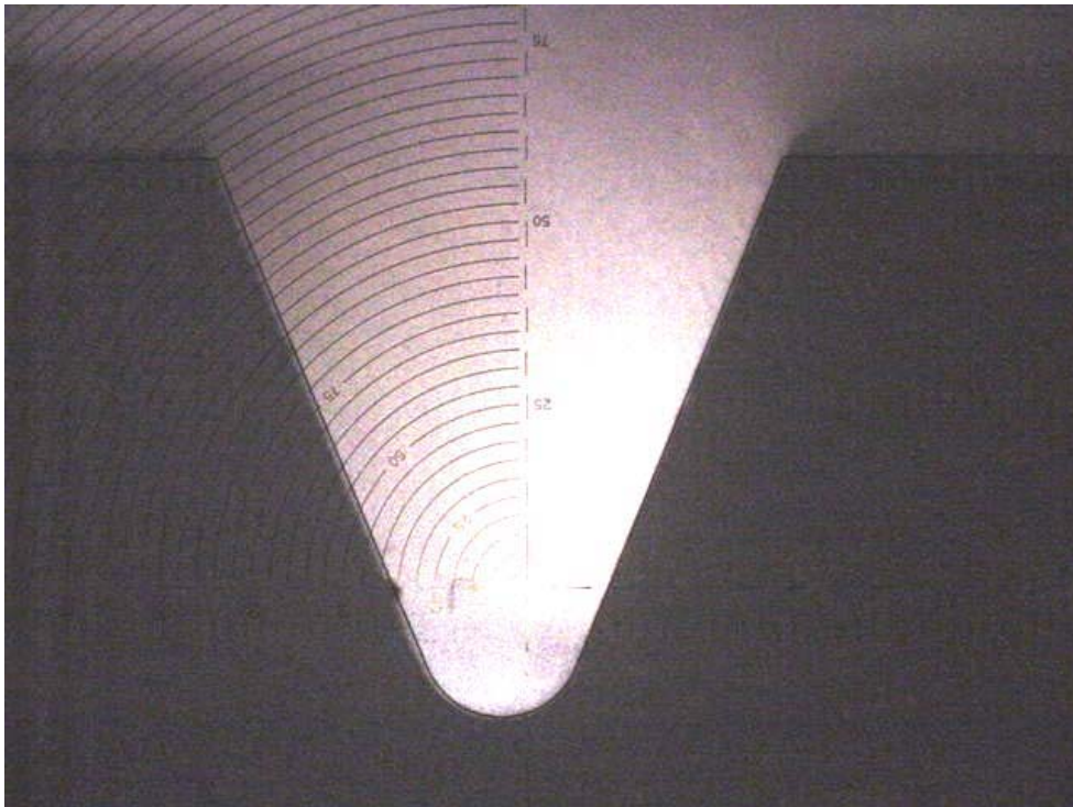
Figure 5.4 Notch of Charpy specimen fabricated by MDOT machinist
