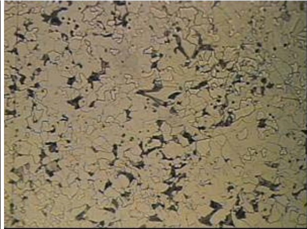
Figure 3.17 Microstructure of heated and unheated portions of the Lansing Road Bridge
