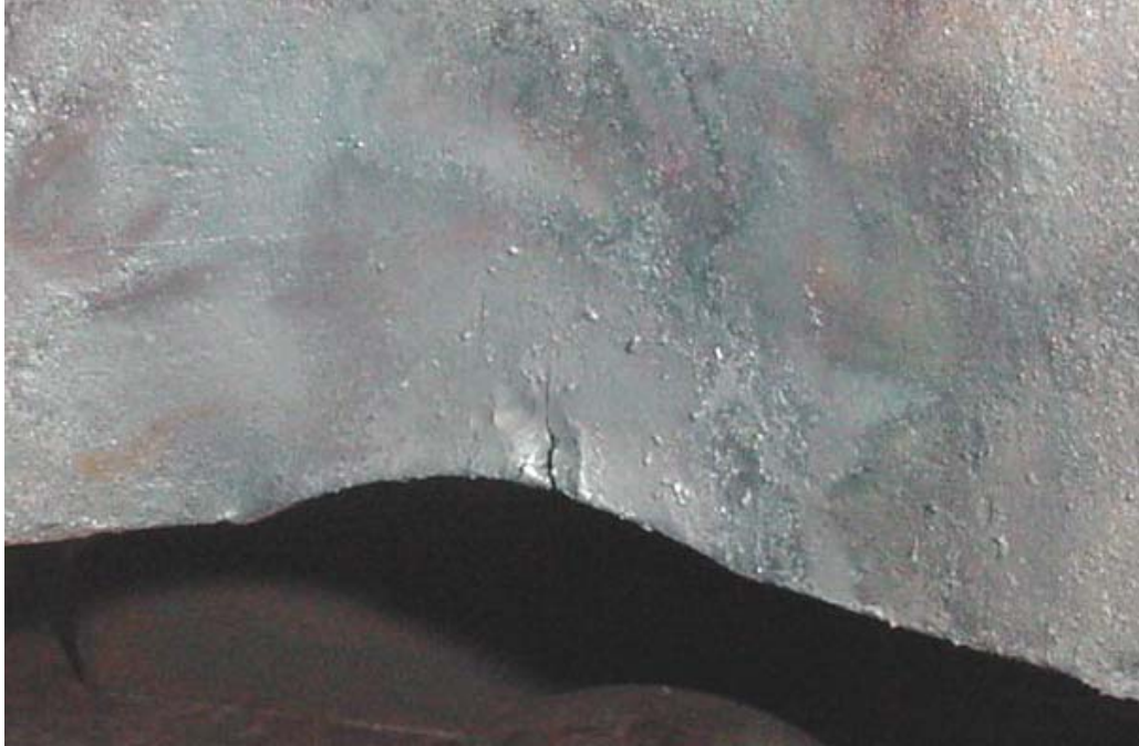
Figure 8.24 Fracture of the material at the buckled location of the front flange of A7-Beam 2
