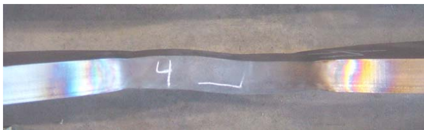
Figure 5.29 Test area of Specimen A588-60-25-4 after experimental investigations
