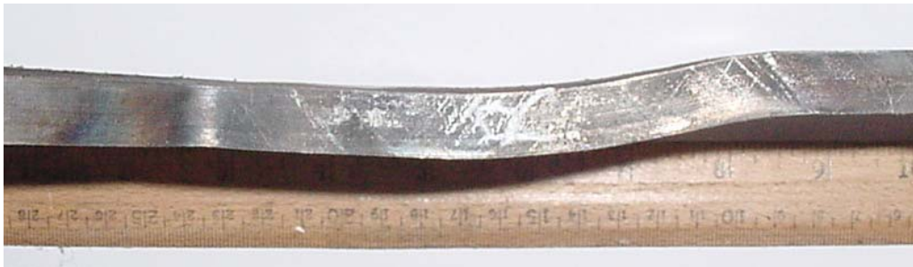
Figure 5.48 Induced curvature in the test area of Specimen A7-90-40-1
