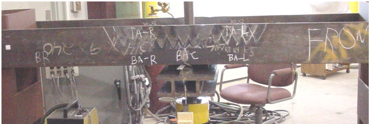
Figure 8.59 Front view of A588-Beam 2 after three damage-repair cycles
