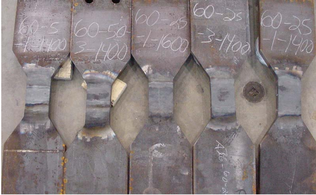
Figure 5.65 Frontal view of overheated A36 specimens after experimental investigations
