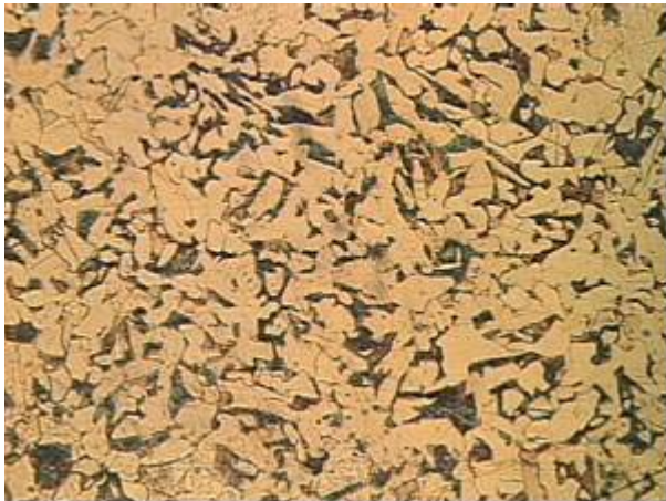
Figure 3.16 Microstructure of heated and unheated sections of the Lake Lansing Road Bridge
