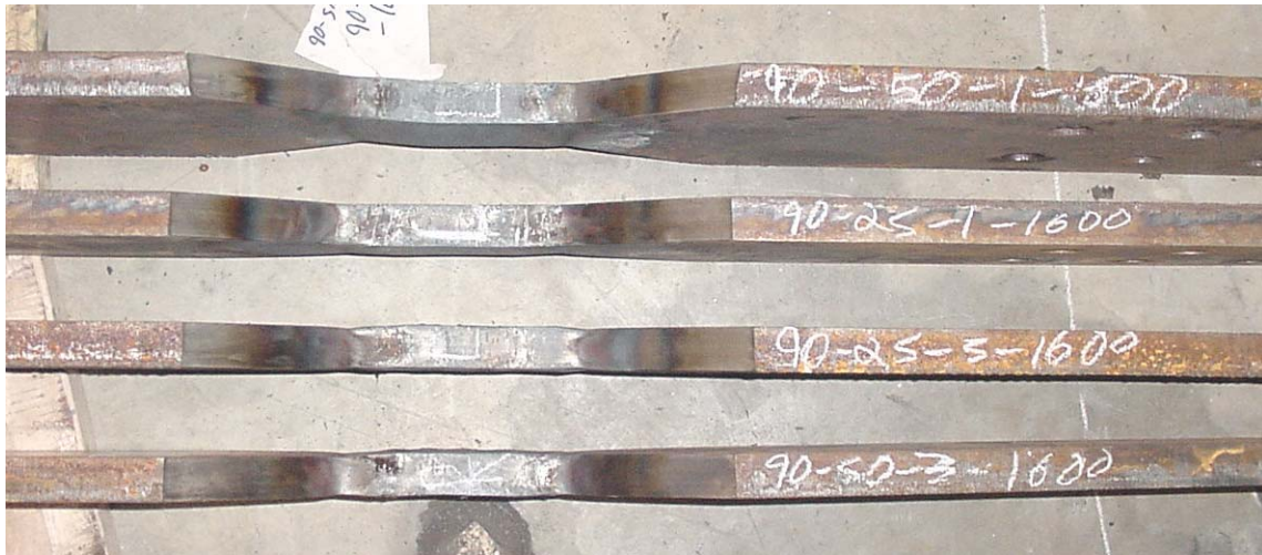
Figure 5.67 Side view of overheated A36 specimens after experimental investigations
