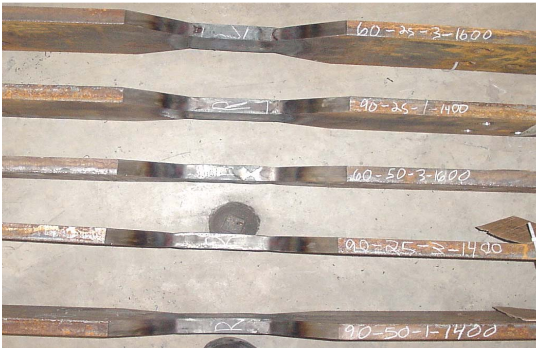
Figure 5.66 Side view of overheated A36 specimens after experimental investigations
