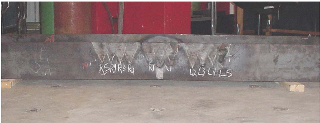
Figure 8.31 Frontal view of A36-Beam 1 after experimental investigations
