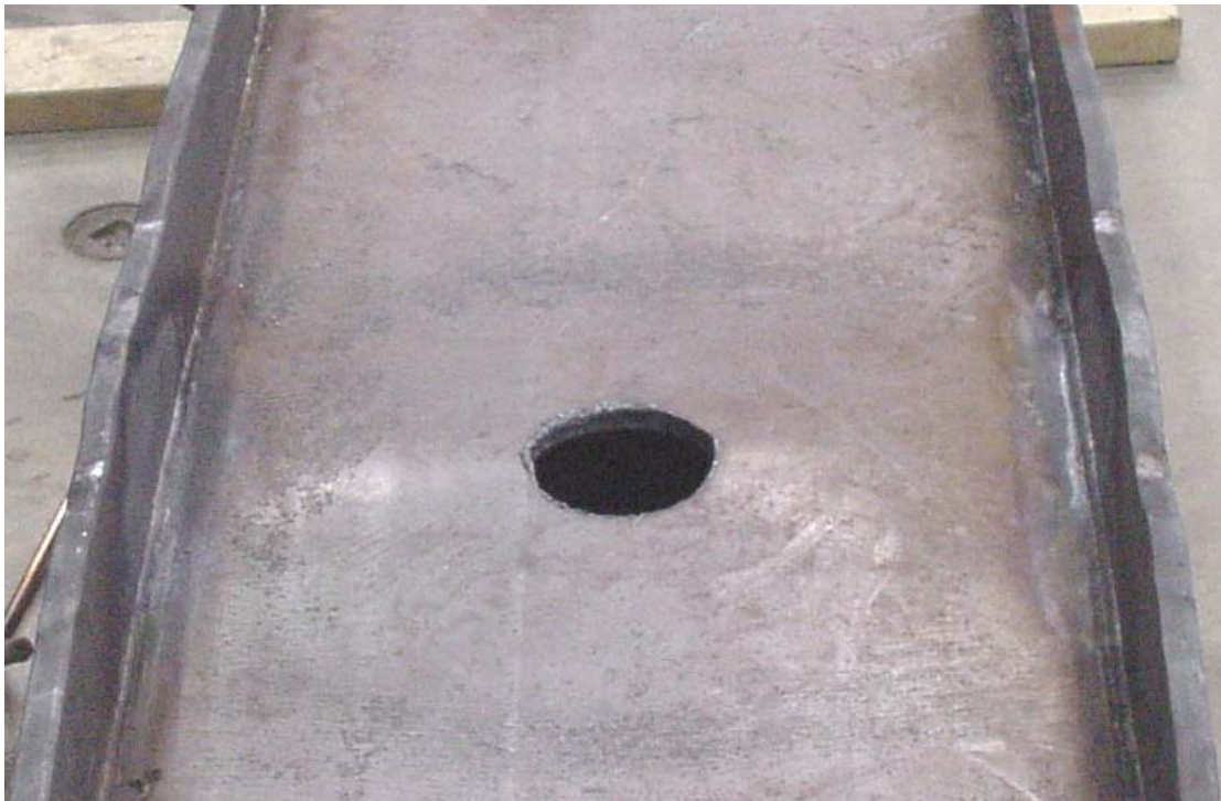
Figure 8.32 Lateral displacement of A36-Beam 1 after experimental investigations
