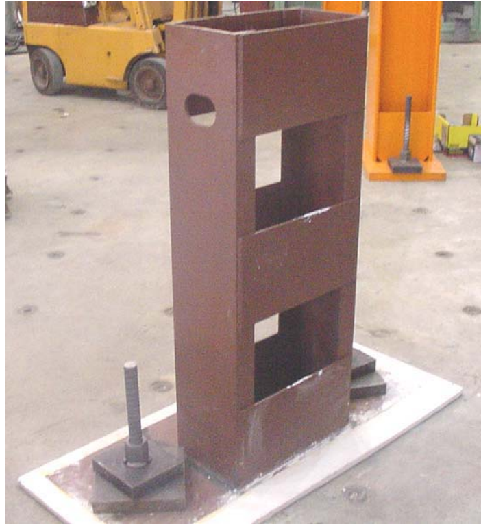
Figure 7.5 Photograph of the roller support column
