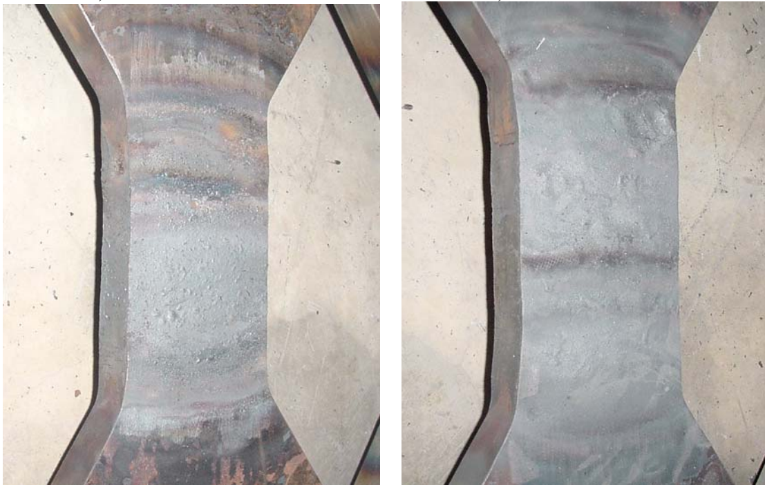
Figure 5.68 Surface conditions of A36 steel after being repaired with T_{max} = 1600 °F
