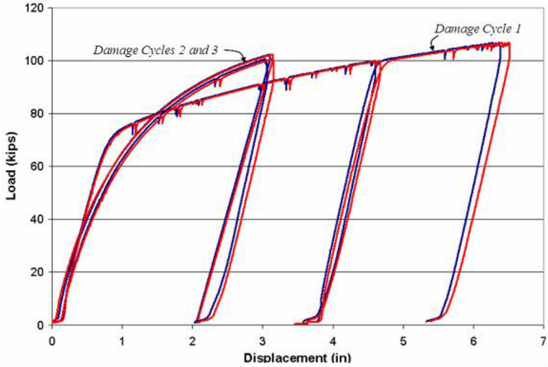
Figure 8.54 Load-displacement behaviors of all three damage cycles of A588-Beam 1
