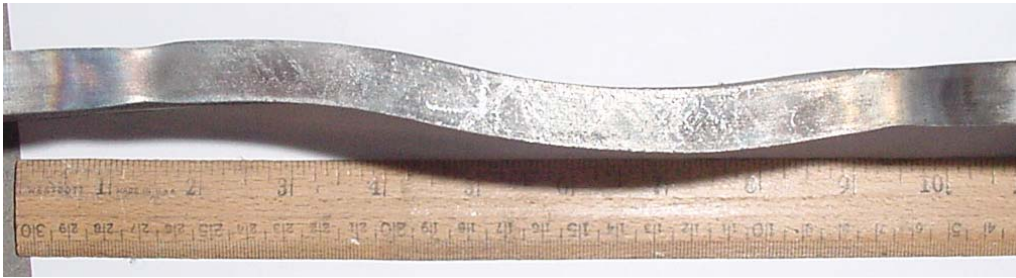
Figure 5.47 Induced curvature in the test area of Specimen A7-90-25-3
