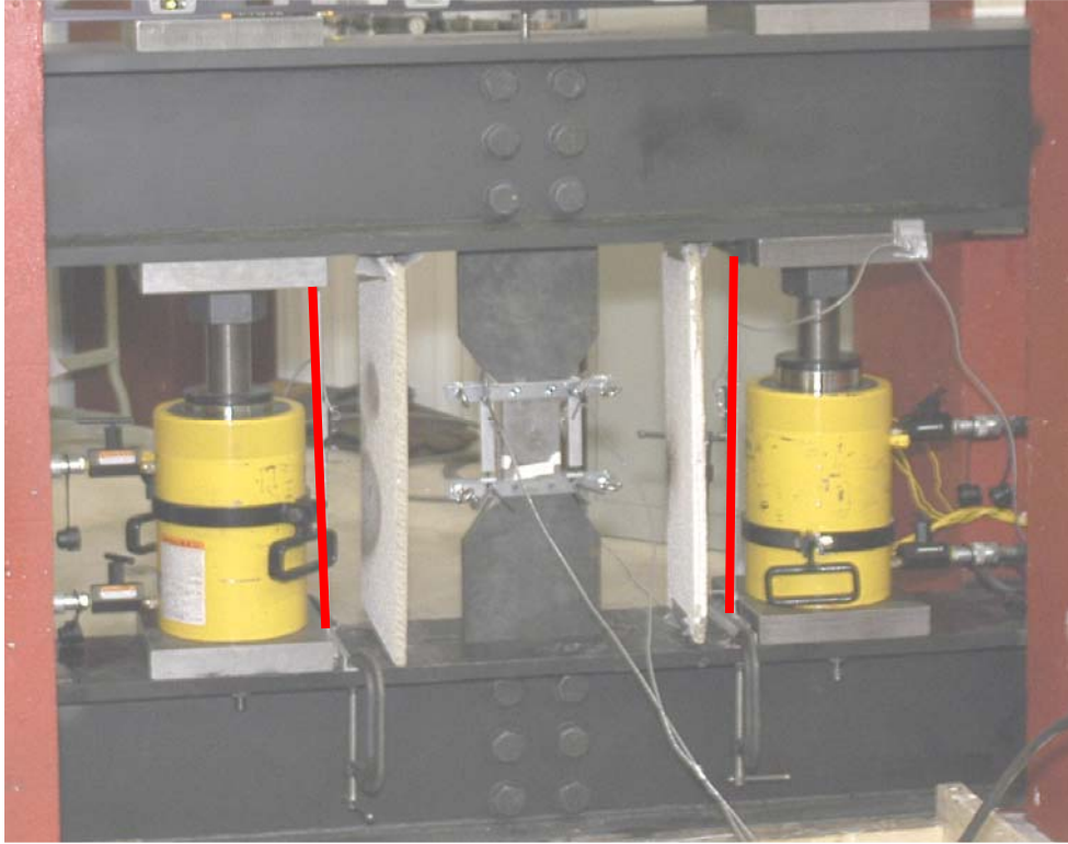
Figure 4.35 1.5 in. displacement transducer locations in respect to the test setup
