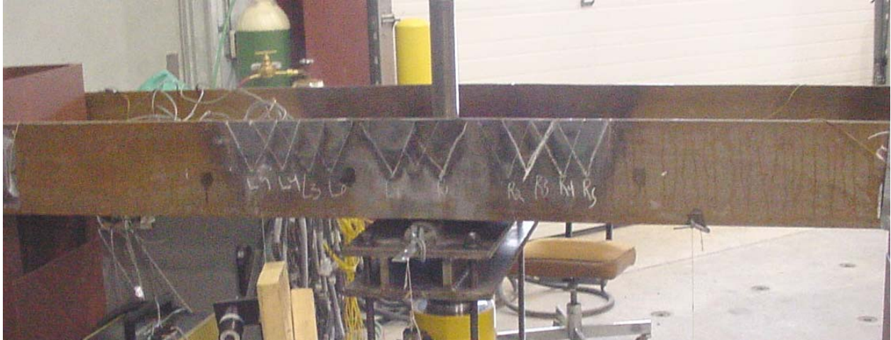
Figure 8.10 Front view of A7-Beam 1 after experimental investigations
