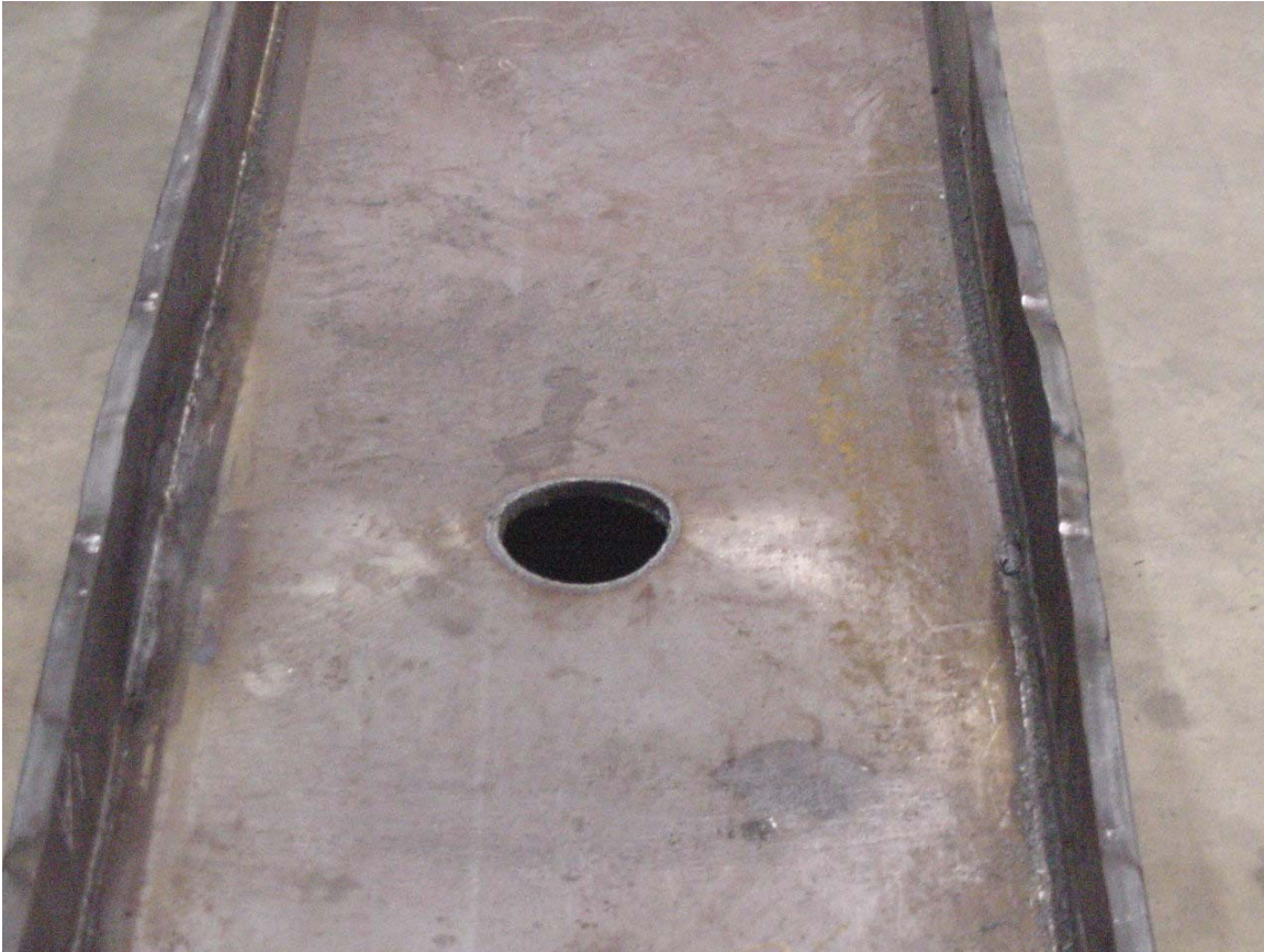
Figure 8.41 Lateral displacement of A36-Beam 2 after experimental investigations
