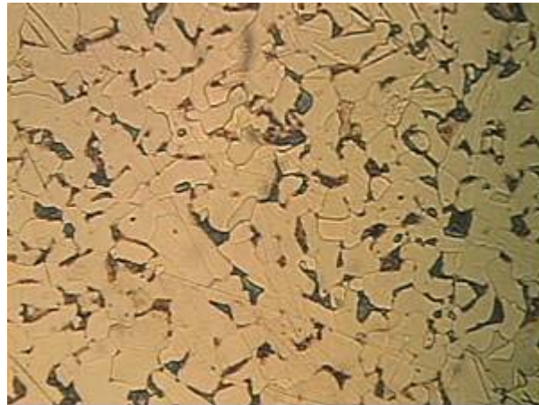
Figure 3.16 Microstructure of heated and unheated sections of the Lake Lansing Road Bridge
