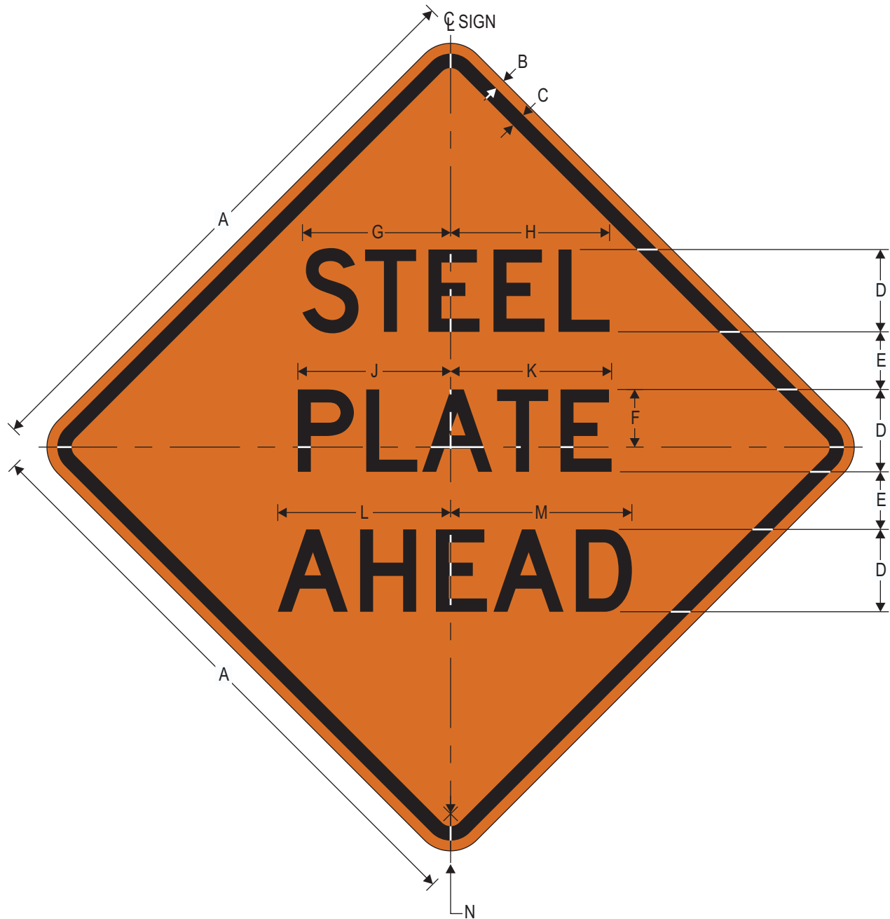
W8-24 STEEL PLATE AHEAD
