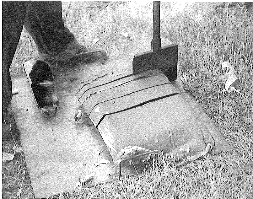
Figure 3. Hot steel spade being used to cut seal into thin slices preparatory to melting. Note steel plate for preventing contamination of seal.
