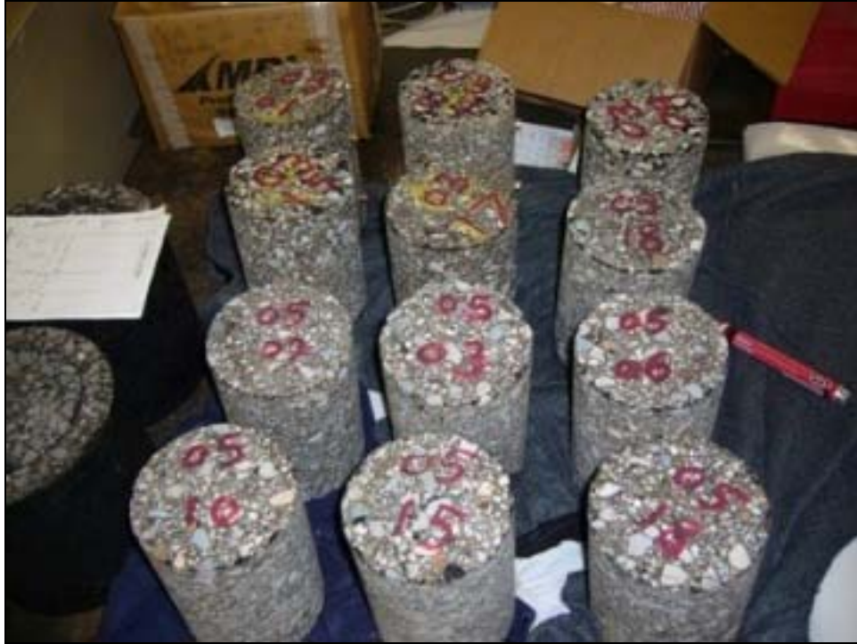
Figure 8 Asphalt Mixture after Cutting and Coring process
