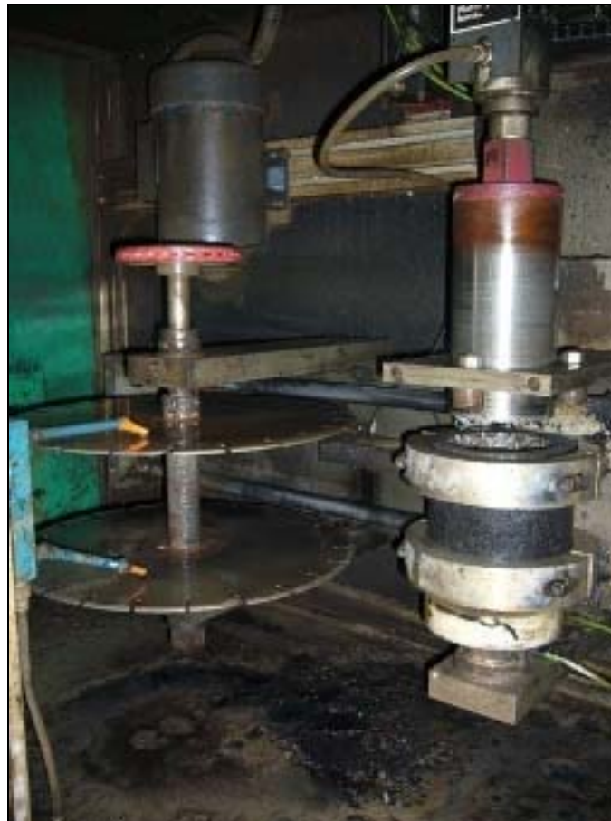
Figure 7 Cutting and Coring Process
