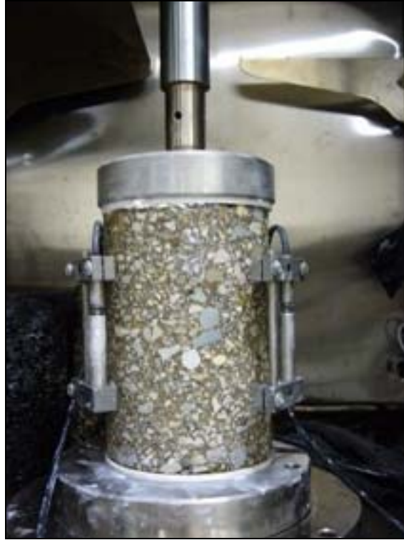
Figure 11 Dynamic Modulus Test Setup
