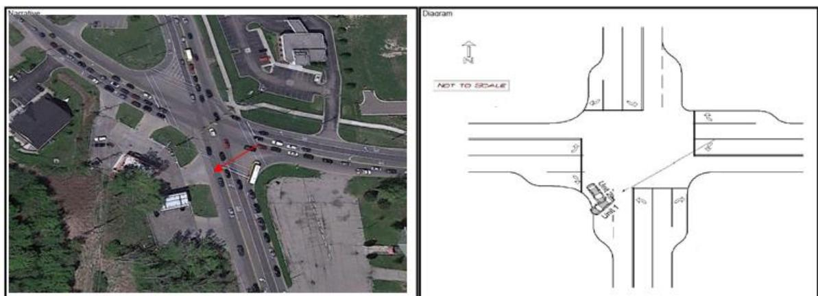
**Figure 4.13 Example of improper left turn maneuver at skewed intersection which resulted to a crash**
