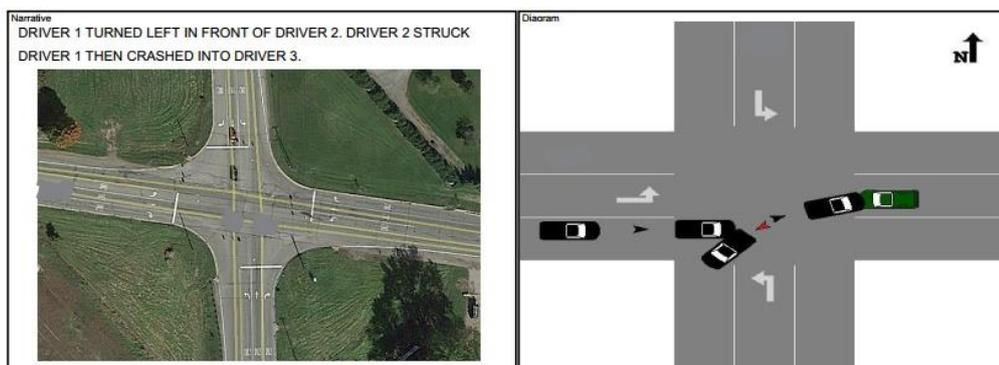
**Figure 4.16 Example of crash type that can be avoided by providing left-turn offset**
