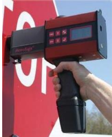
A retroreflectometer can be used to determine if a sign meets or exceeds the minimum required retroreflectivity level.
