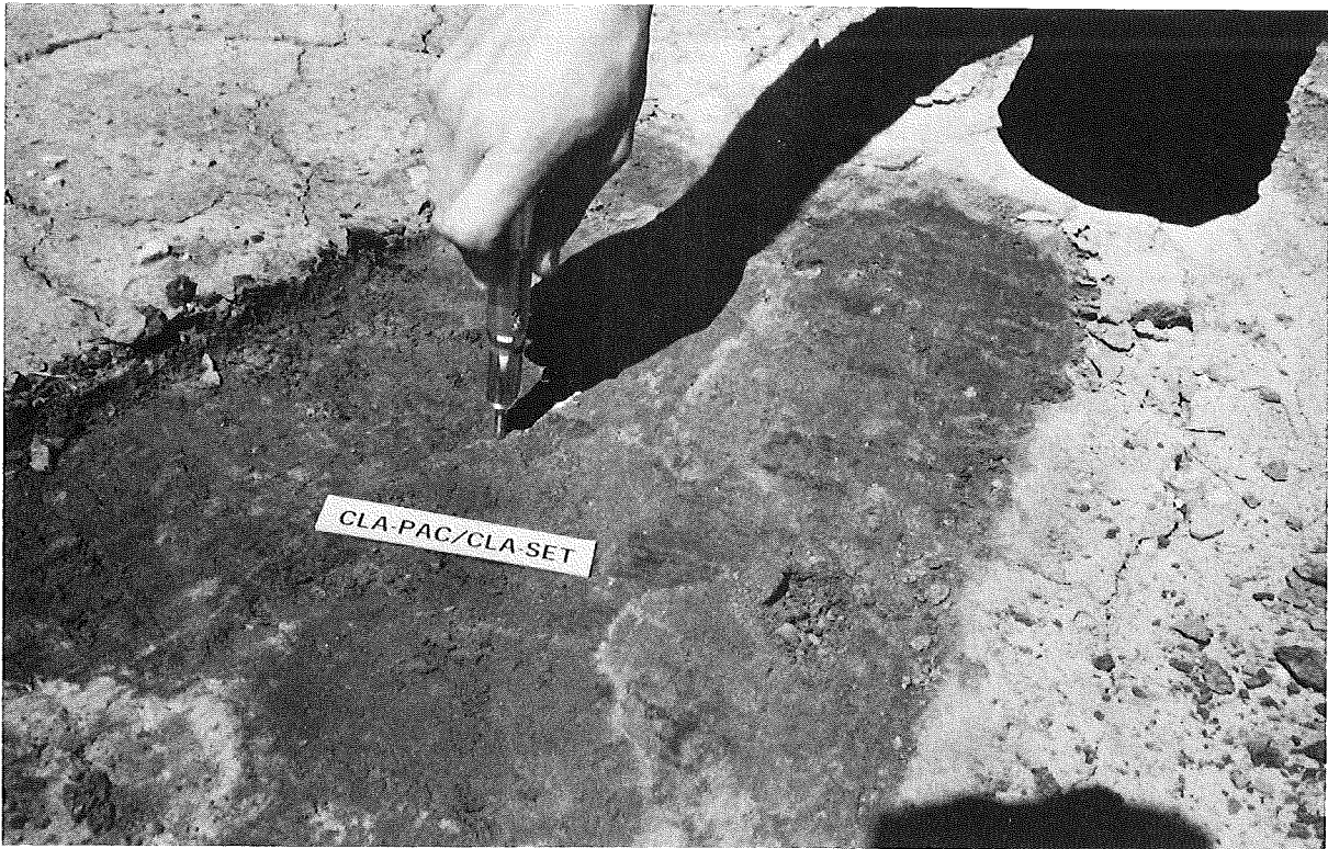
Figure 6. Penetration testing of the test areas.
