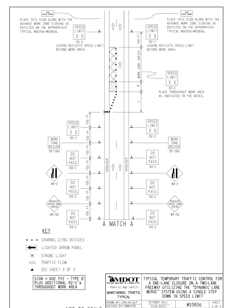
NOT TO SCALE | CHECKED BY: BMM: CRB | PLAN DATE: | FILE: PW RD/TS/Typicals/Signs/MT FWY/M1080a.dgn
