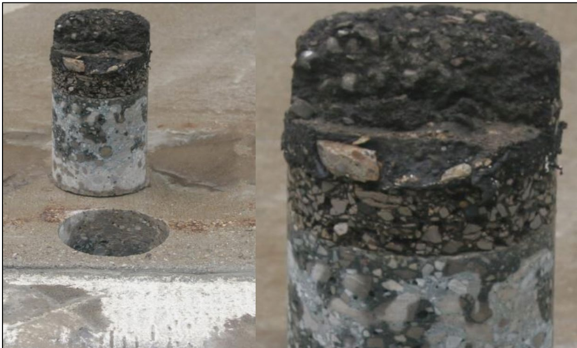
Figure A17. MDOT Report # RC-1574, Figure A3, Dense-graded HMA Not Milled Off During Construction
