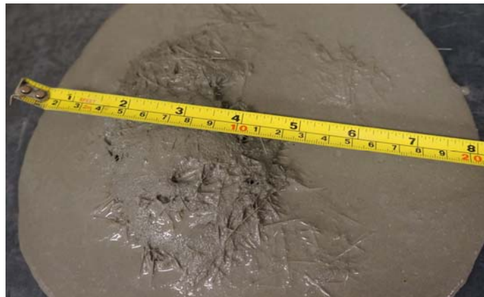
Figure 5-18 The segregation caused by high dose of HRWR
