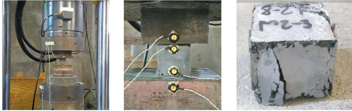
Figure 4-3 Testing set-up for compression tests of cube specimens
