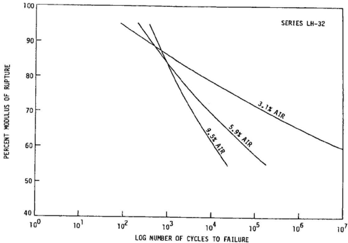
Figure 2.3. Effect of Air Content on Fatigue Life (Klaiber and Dah-Yin Lee)
