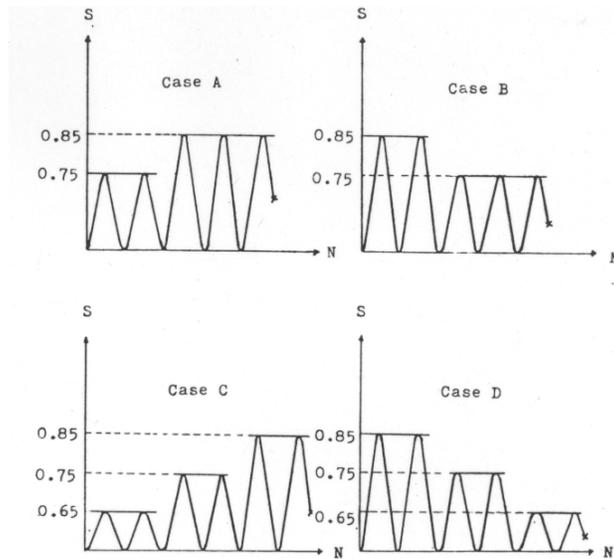
Figure 2.2. Types of various-amplitude fatigue loadings (Oh, 1991)
