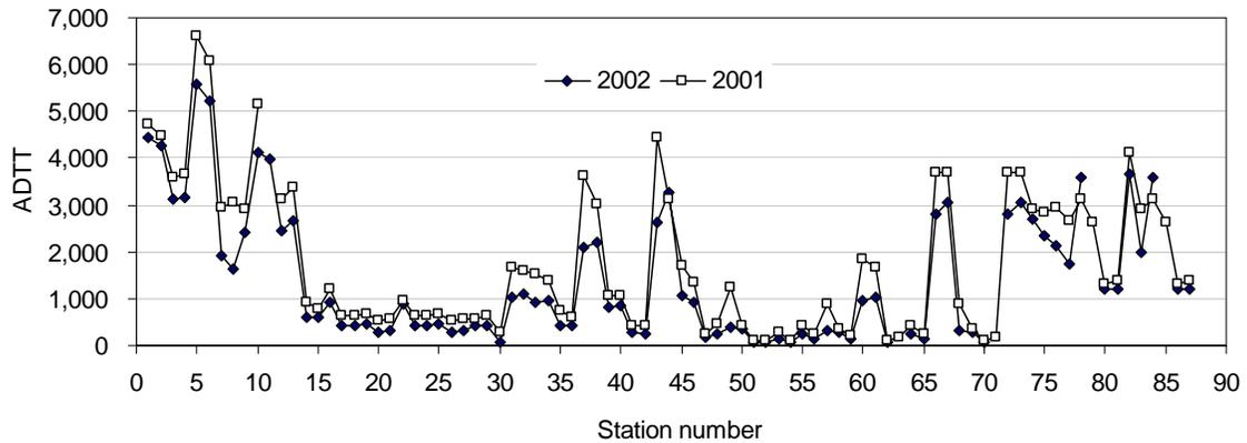
Figure 3.1. Comparison between 2001 and 2002 total average daily truck traffic by station
