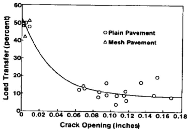
Figure 2.7. Effect of Crack opening on LTE (Colley and Humphrey, 1967)
