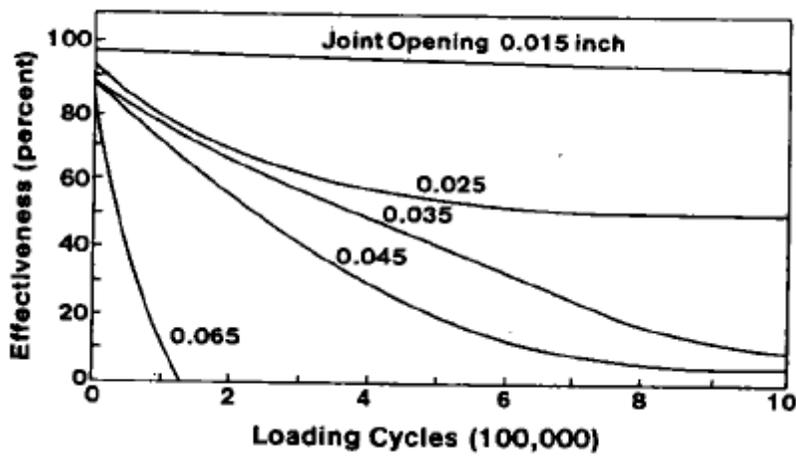
Figure 2.9. Joint Efficiency vs. Loading Cycles for different crack widths (Colley and Humphrey)
