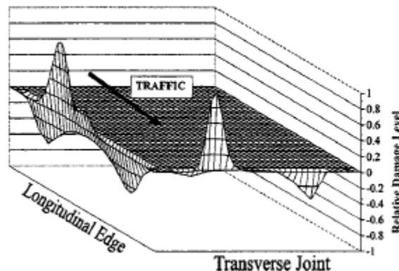
Figure 2.5. Relative damage levels using stress range approach along top and bottom of slab with effective built-in temperature difference of  $-30^{\circ}$  Fahrenheit (Hiller and Roesler)
