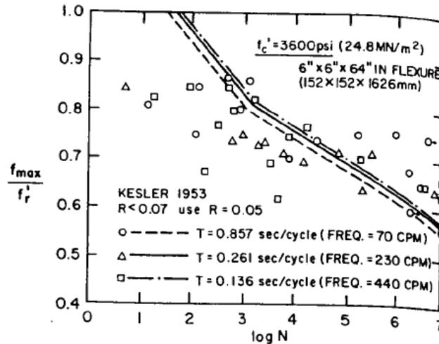
Figure 2.4. Comparison of Hsu Model with Previous Fatigue Data (Hsu)
