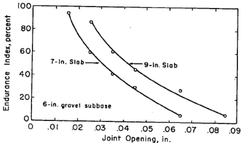
Figure 2.10. Joint Efficiency vs. Joint Opening for different slab thicknesses (Colley and Humphrey)
