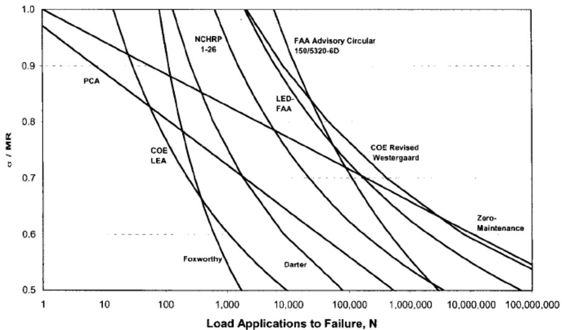
Figure 2.6. Comparisons of Fatigue Models (Smith and Roesler, 2003)
