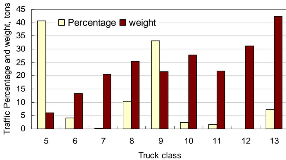
Figure 3.4. Weight and percentage of FHWA truck classes
