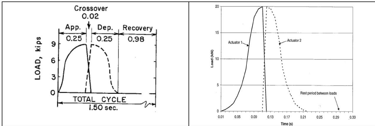
Figure 2.8. Typical load waveforms for dynamic loading (Colley and Humphrey; Hanekom, Horak and Visser)
