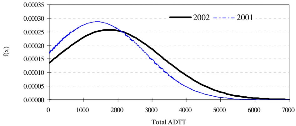
Figure 3.2. Comparison between 2001 and 2002 total average daily truck traffic by traffic distribution
